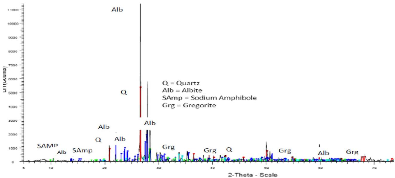
Fig. 4 Graph of representative XRD results for soils collected over gneiss basement at 0.5 m depth
