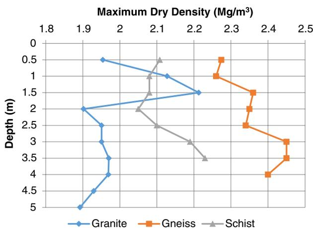
Fig. 12 Variation of maximum dry densities with depth
