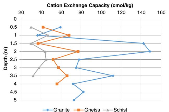
Fig. 7 Variation of cation exchange capacity with depth
