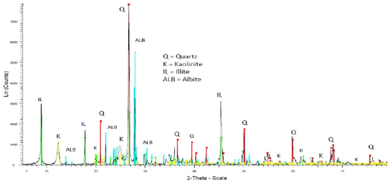
Fig. 3 Graph of representative XRD results for soils collected over schist basement at 0.5 m depth
