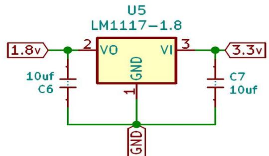
Figure 4: Voltage regulator circuit diagram
