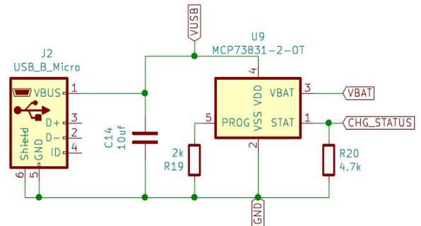
Figure 3: USB LiPo battery charging circuit
