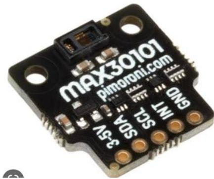
Figure 5: MAX30101 HR and BP sensor
