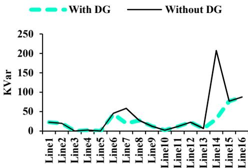
Fig. 3 Reactive line losses with and without DG on test network
