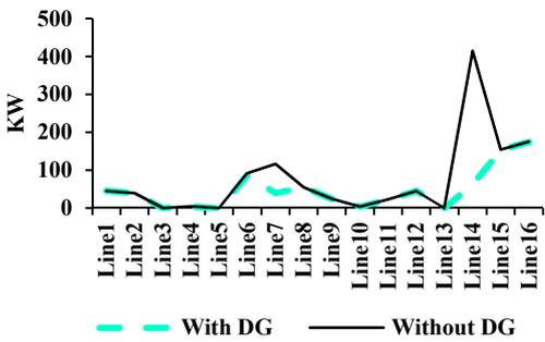
Fig. 2 Real line losses with and without DG on test system
