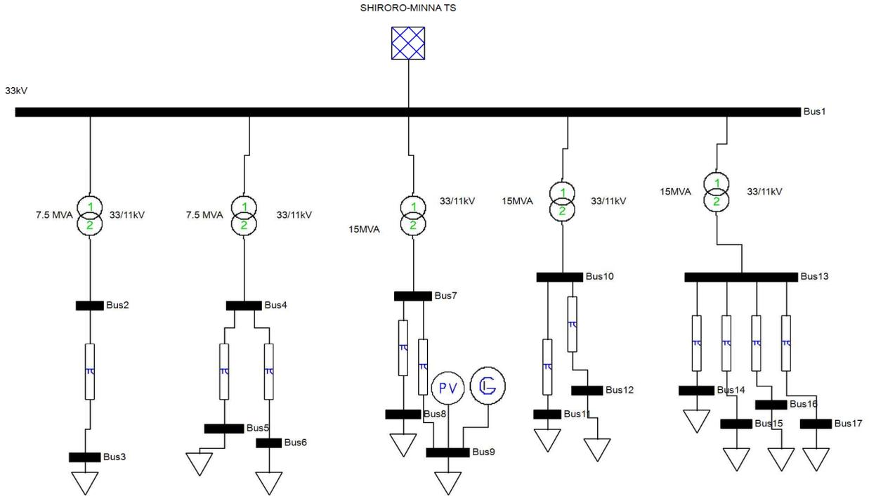
Fig. 1 PSAT model of test network with DG
