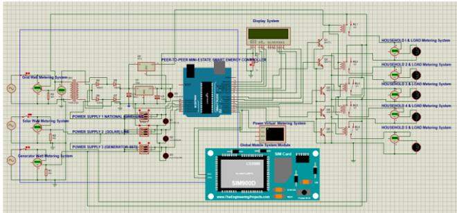
Figure 2: Proposed circuit diagram for Peer-to-Peer Mini-Estate Smart Energy Monitoring and Control Model
