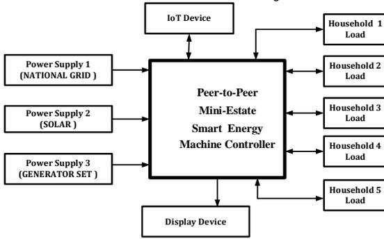
Figure 1: The Integrated Energy Architectural Model controller with relays, Arduino microcontroller, transistors, IoT device, liquid crystal display, synchronizers and busbar and five detachable households as load centers.
