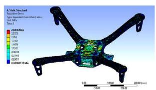
Fig. 5: Frame structure results for stress analysis
