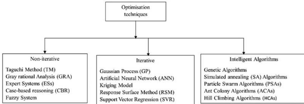
FIGURE 4.—Classification of optimization techniques used for injection molding process.
