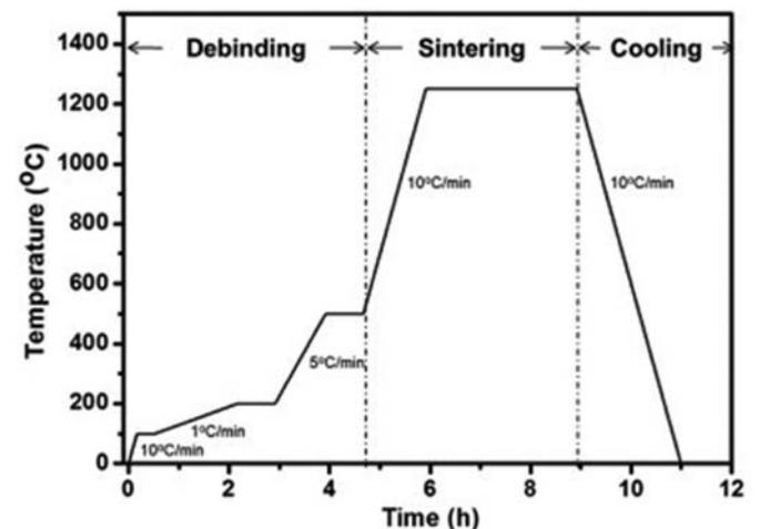
FIGURE 2.—Schematic of the thermal debinding and sintering processes [81].
