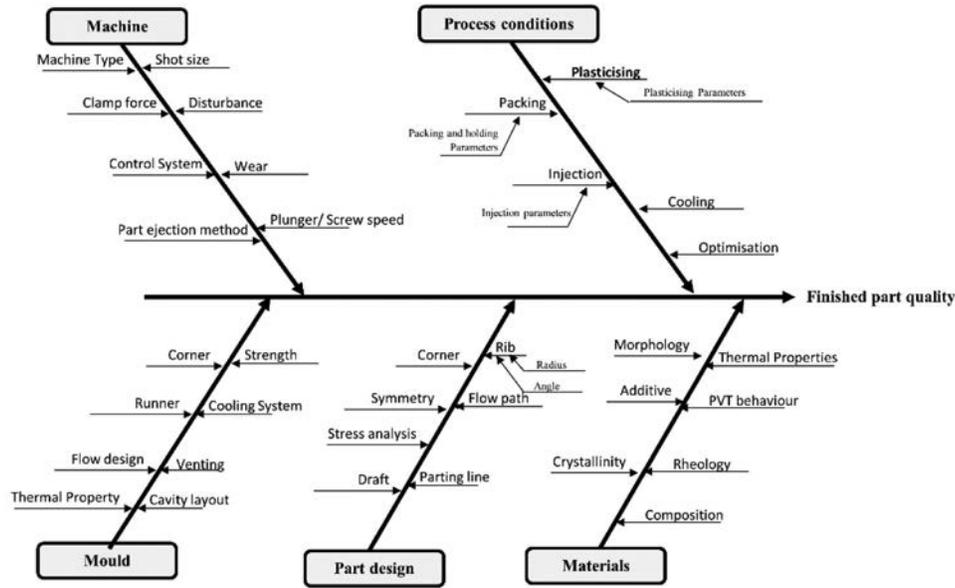
FIGURE 7.—The interactions of critical factors influencing part quality of injection molding products.
