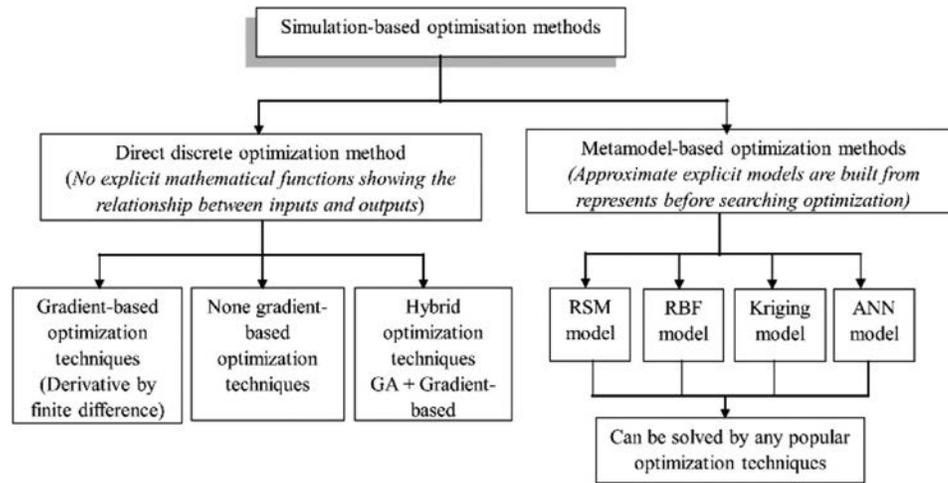
FIGURE 6.—Classification of simulation-based optimization techniques [1].
