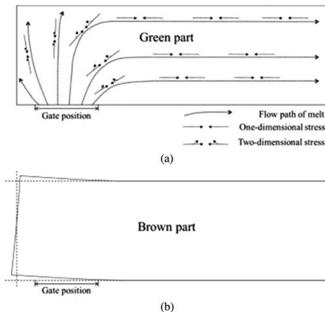
FIGURE 3.—(a) Possible flow path of melt in mold cavity generating internal stresses because of frozen-in orientation and (b) distortion of brown part due to stress relaxation [27].
