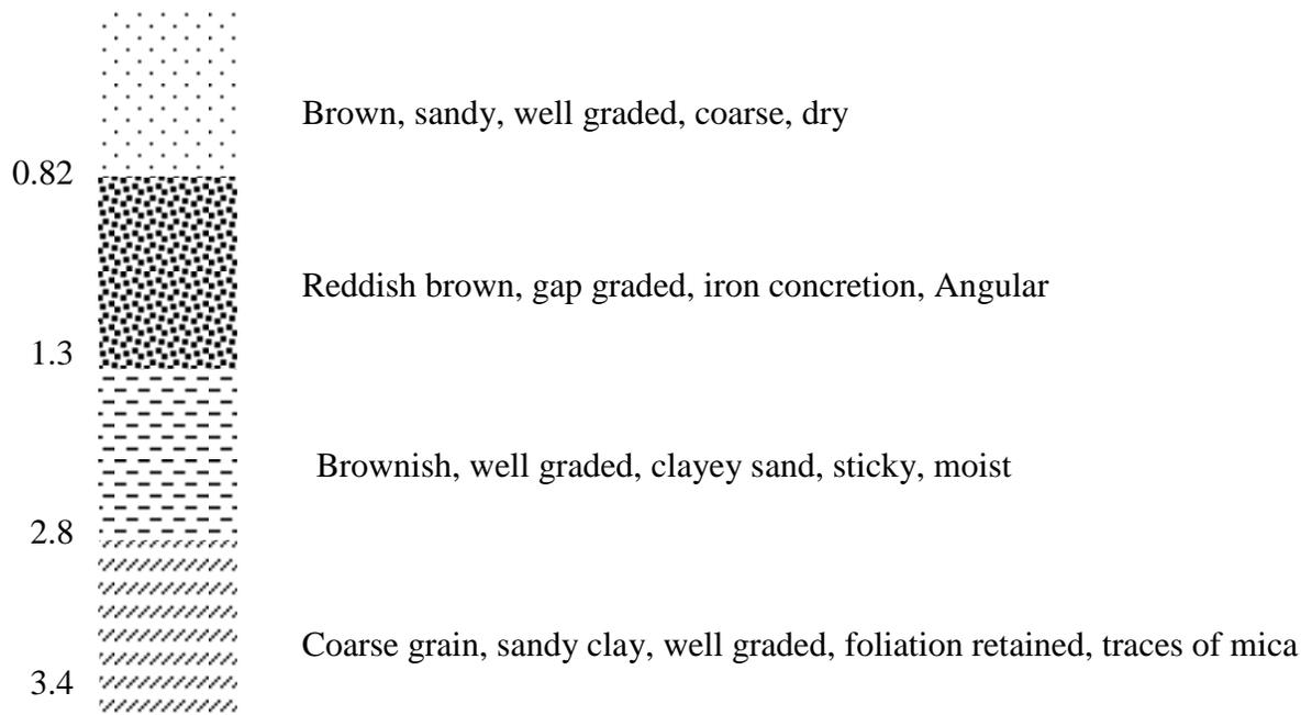
Figure: 4.2 Typical Soil Profile at Eyenkorin Bridge along the road
