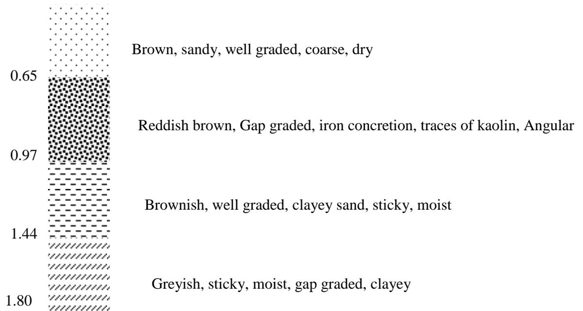
Figure 4.2 Typical Soil Profile at Lautech junction along the Road
