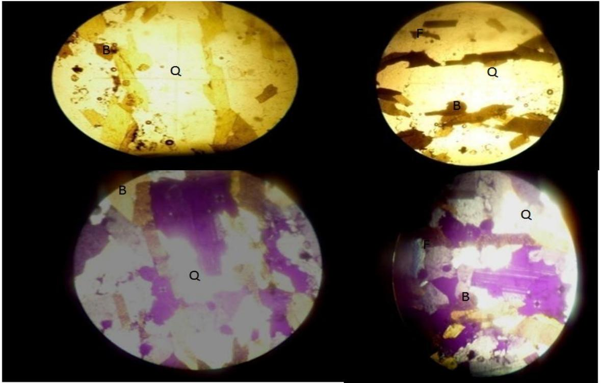
PLATE: III Mineral assemblage in thin section of the Migmatite (B= Biotite, Q= Quartz F= Feldspar; top two, under plane polarized light and last two cross polarized light)
