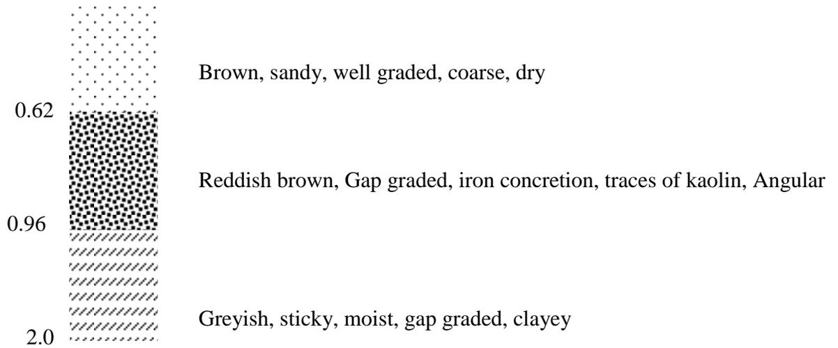
Figure 4.2 Typical Soil Profile at location Aduka and Gambri along the Road
