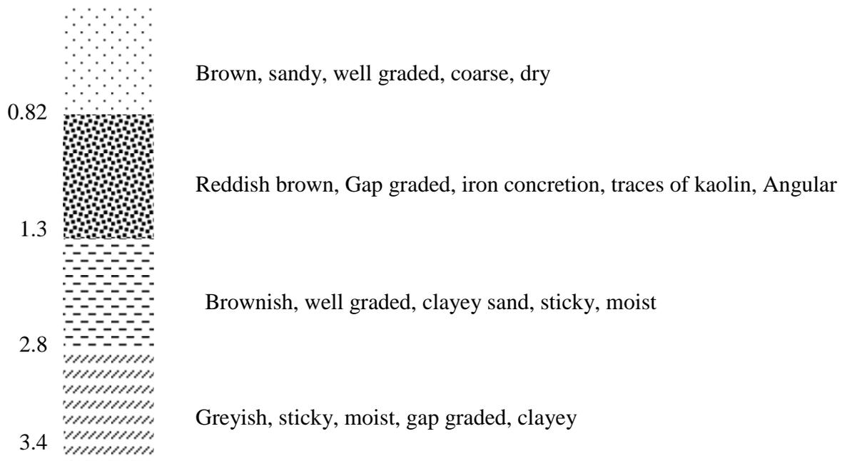
Figure 4.2 Typical Soil Profile at Araromi along the Road
