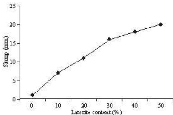
Figure 1: Slump of laterized concrete vs laterite .
