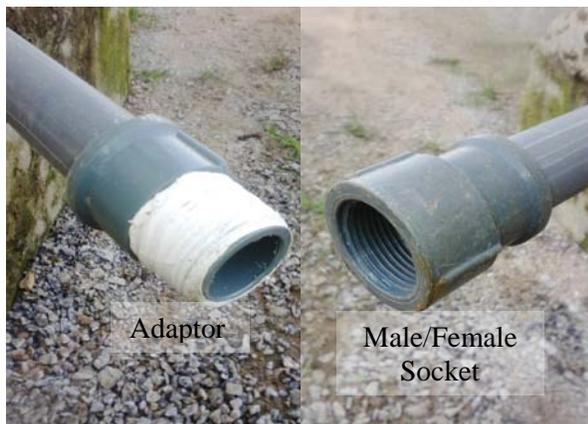
Plate II: Picture of pipe connectors
