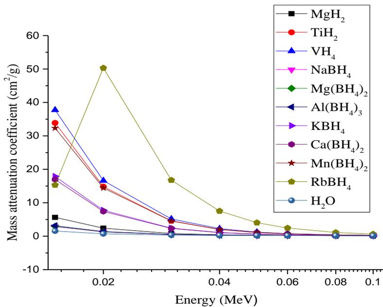
Figure 3a. Mass attenuation Coefficients of the substances in the low energy region.
