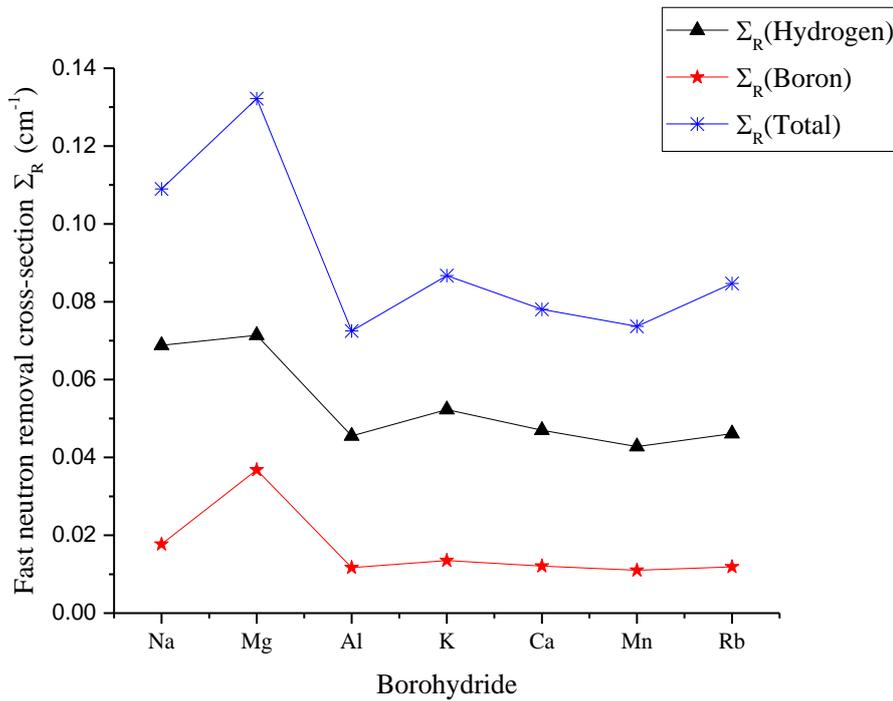
Figure 2. Fast neutron removal cross section for the borohydrides and boron and hydrogen content.
