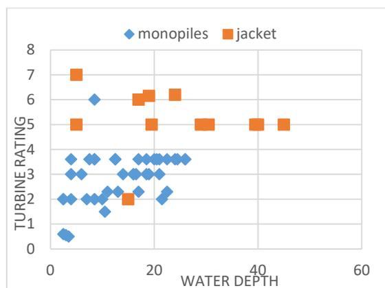
Figure 1. Graphical plot of turbine ratings (in MW) against water depths (in m) for OWTs supported on monopile and jacket foundations between years 2000 and 2018.
