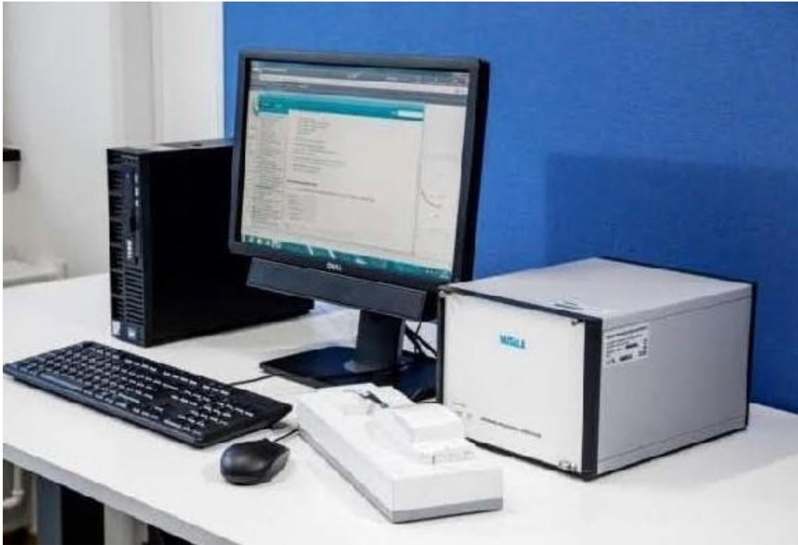
Figure 1: DigiCORA and Radiosonde sounding system from [7]
