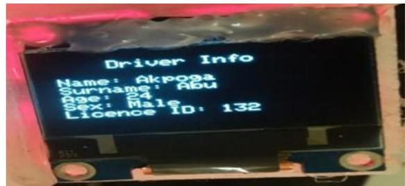
Figure 4. OLED Display of a Registered Driver's Information
