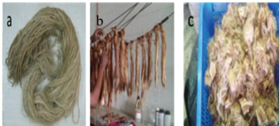
Fig. 1. Kenaf fibre: (a) Untreated long curled fibre, (b) drying treated fibre, (c) chopped treated kenaf fibre.
