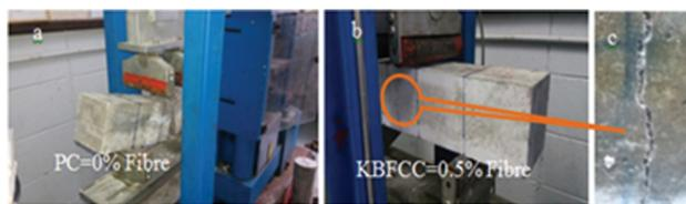
Fig. 4. Failure mode of prism in flexure (a) PC specimen, (b) KBFCC specimen, (c) Kenaf fibre bridging the cracked planes.
