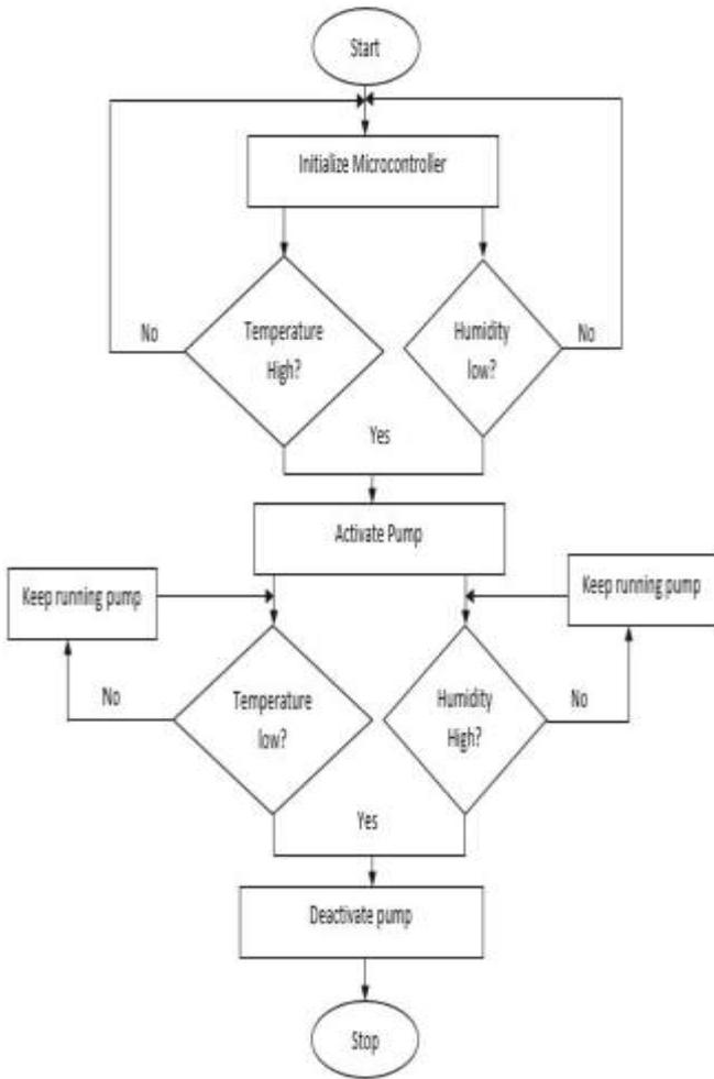
Figure 5: Flowchart of temperature and humidity sensing
