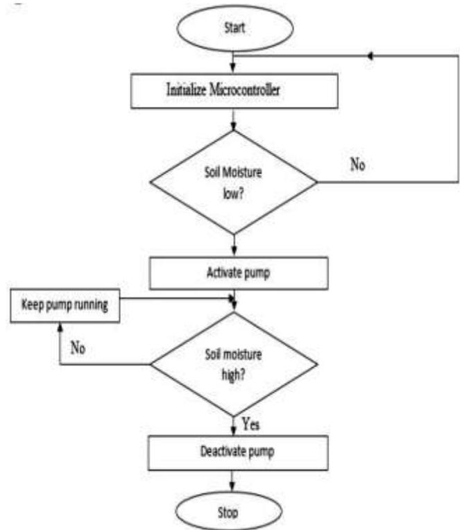
Figure 4: Flowchart of the soil moisture sensing
