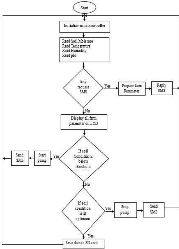
Figure 2: Flowchart of the control system
