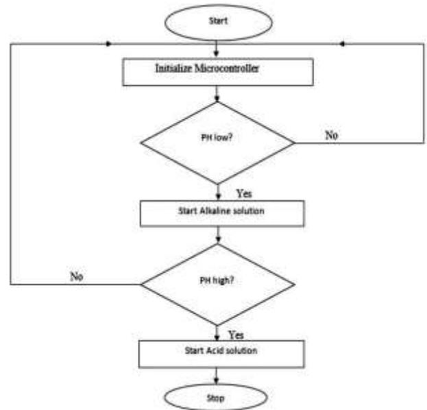
Figure 7: Flowchart of the pH sensing
