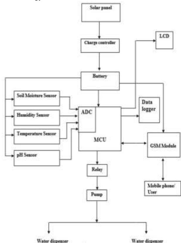
Figure 1: Block diagram of the GSM based irrigation control system
