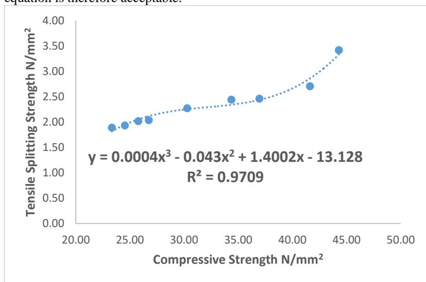
Figure 6: Relationship between compressive and splitting tensile strength.
