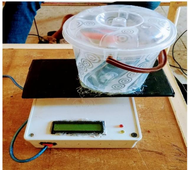
Figure 4: Overall view of fuel adulteration detection system.
