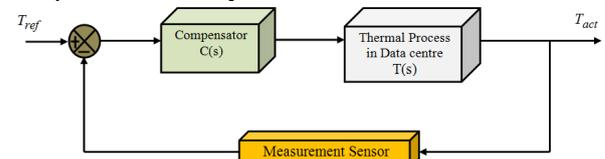
Figure 2: Feedback Network of Temperature Regulating Loop in Data Centre
