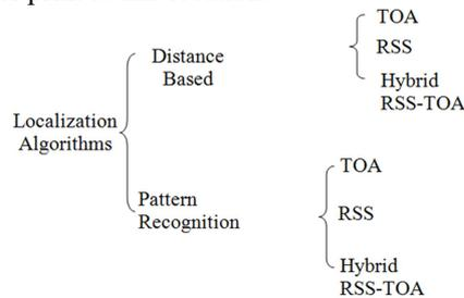
Figure 6: Classification of localization algorithms.
