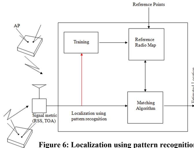
Figure 6: Localization using pattern recognition.
