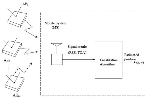
**Figure 1 A Typical positioning System.**
