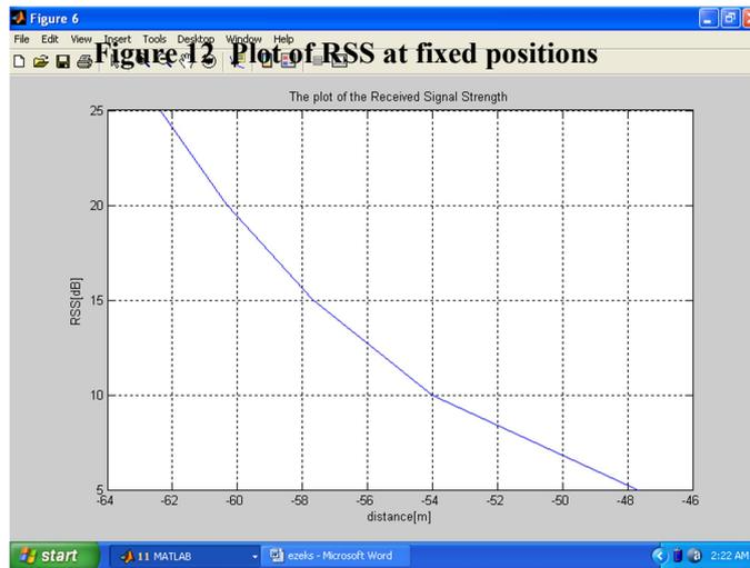
Figure 13 Received Signal Strength against Distance
