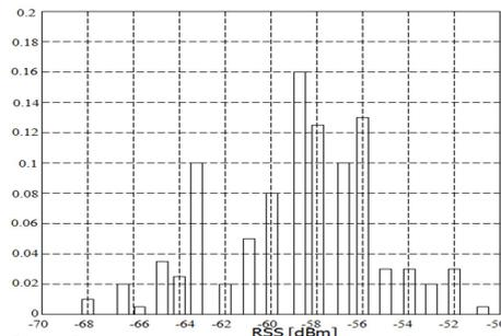
Figure 4: RSS distribution at a fixed location obtained by a WiFi measurement system.
