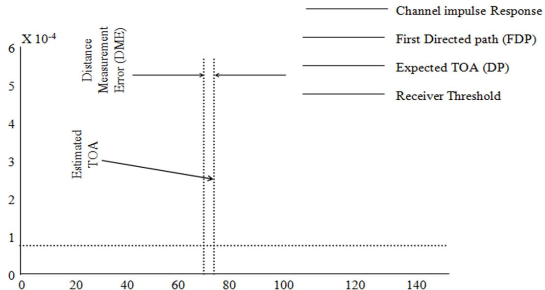
Figure 7: A sample channel impulse response for a 200MHZ system.
