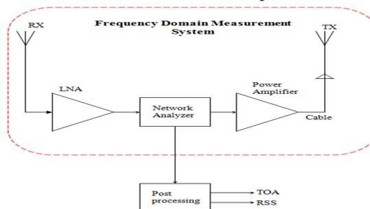
Figure 5: Frequency domain measurement system
