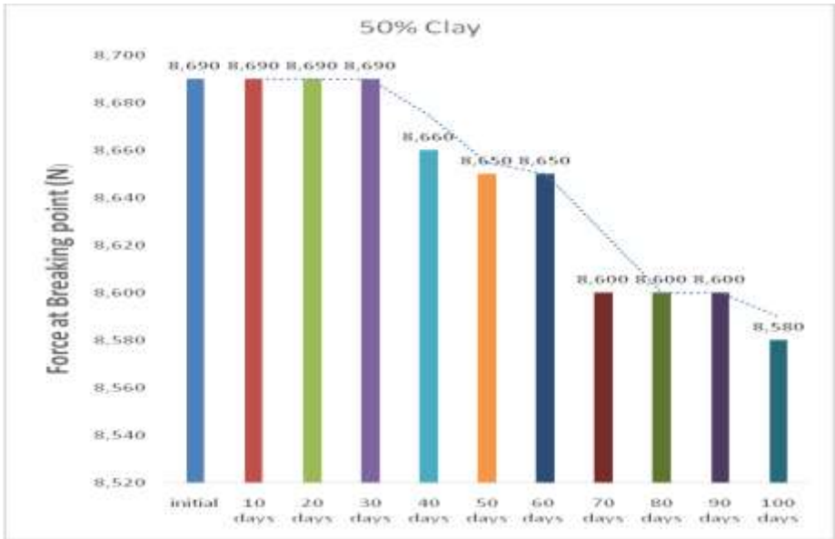
Figure 4.7g: Chart showing forces at breaking points of pavers (Granite 50/50) on activation with weak sulphuric acid for between 0-100days
