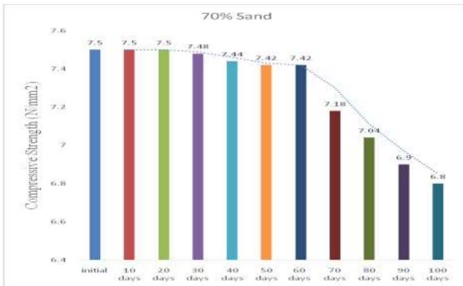
Figure 4.6f: Chart of compressive strengths of pavers (Sand 70/30) on activation with weak sulphuric acid for between 0-100days
