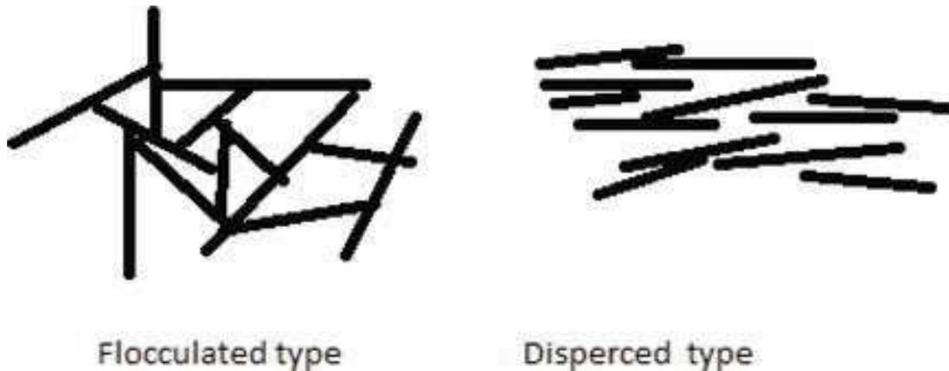
**Figure 2.4:** Clay particle orientations (Advanced soil mechanics by Braja M. Das. 3<sup>rd</sup> edition, 2008)
