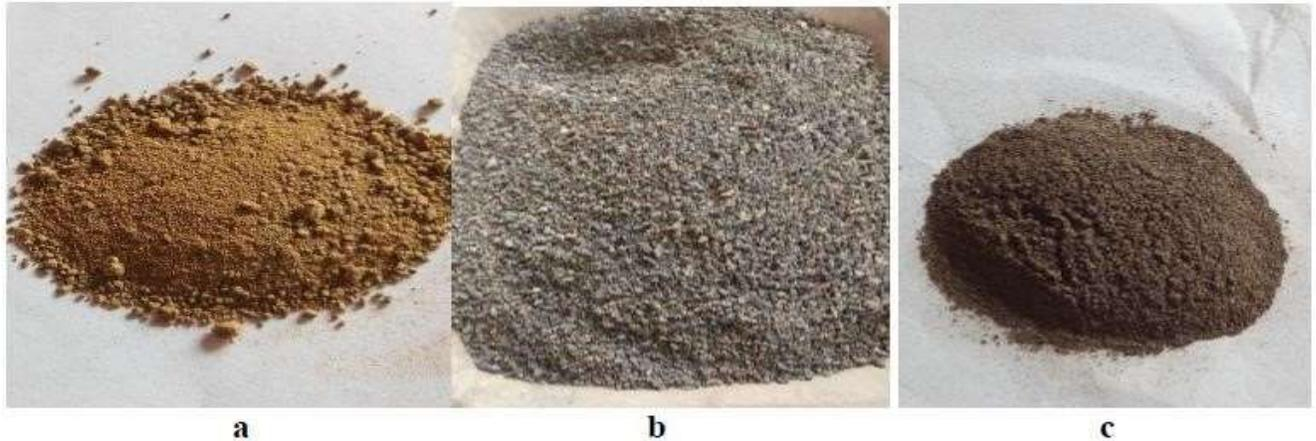
**Figure 3.1:** (a) Clay soil; (b) Unpulverized volcanic ash; (c) Pulverized volcanic ash
