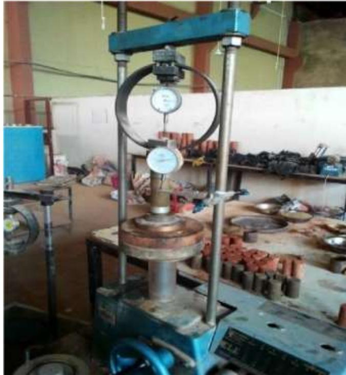
**Plate I:** Unconfined compressive strength test
