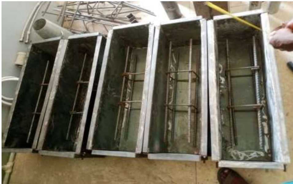
Plate III: Steel moulds fabricated in the laboratory
