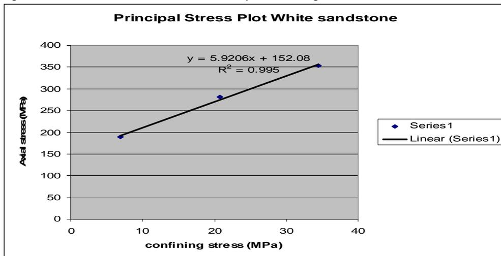
Figure 2: Principal stress plot for Clashach (white) sandstone discrete failure mode
