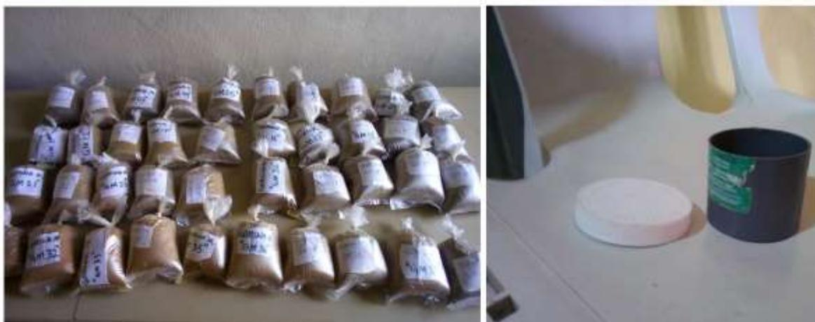
**Plate III:** Packaged 500 g samples and the detector volume-sized plastic container
