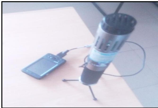
Plates XV: Probe Toxic Gas Analyser Model TG/501
