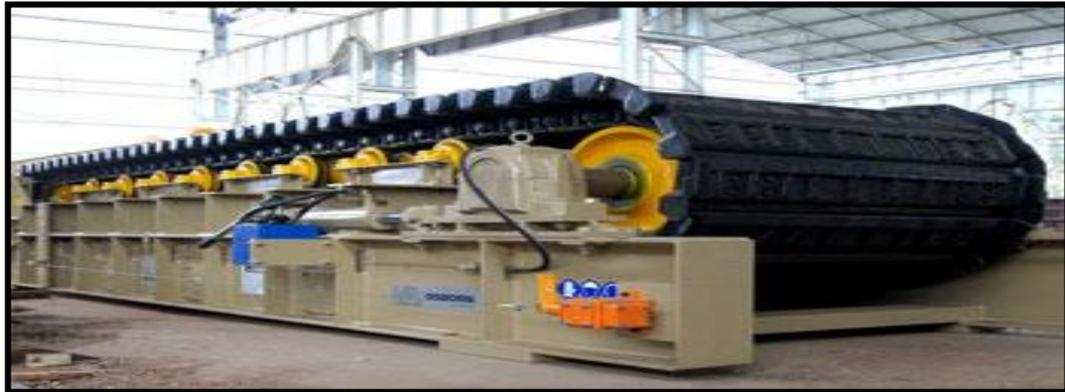
Plate V: BWZ Series Heavy Duty Apron Feeders
