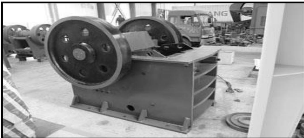
Plate II: PE Jaw Crusher
