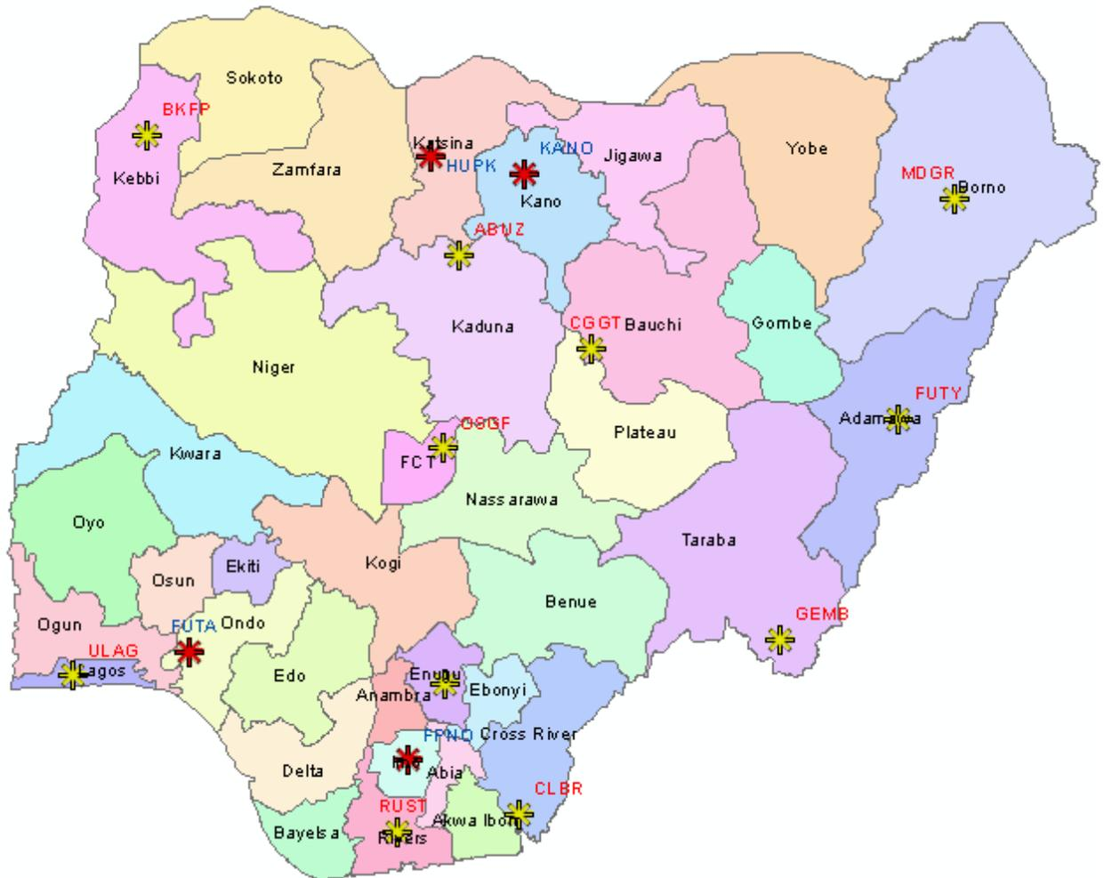
Figure 2.6: Distribution of the NIGNET stations. Yellow – stations already installed (December 2009). Red – stations being installed in January/February 2010.
