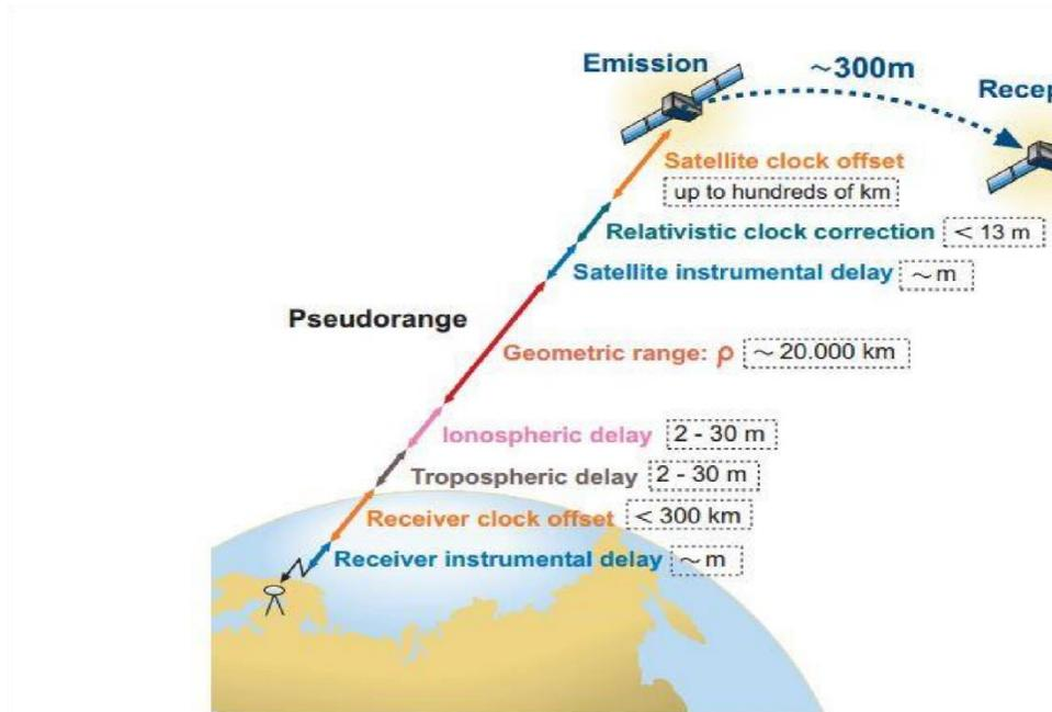
Figure 2.4: Reception and emission of satellite signals with the errors in observables
