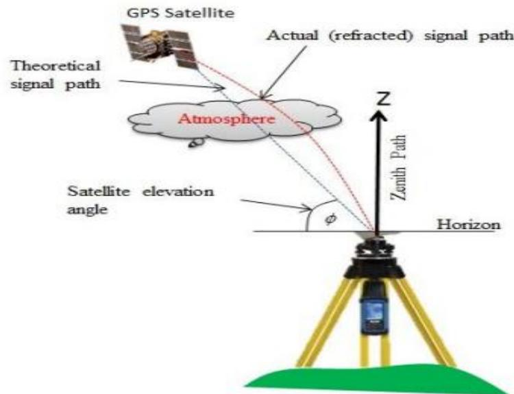
Figure 2.1: Atmospheric effect on GPS signal
