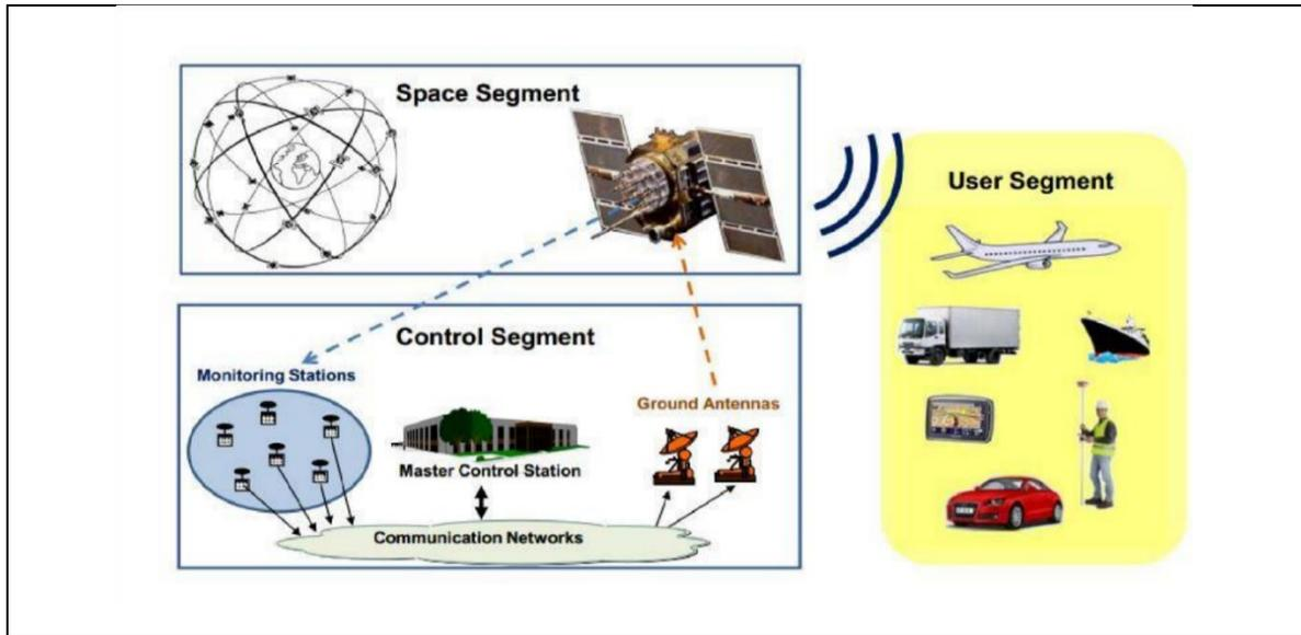
Figure 2.3: GNSS Architecture and segments
