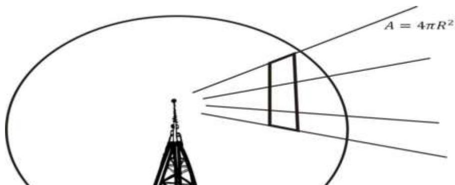
Figure 2.1: An isotropic antenna radiating EMF (Aliyu *et al.*, 2018).
