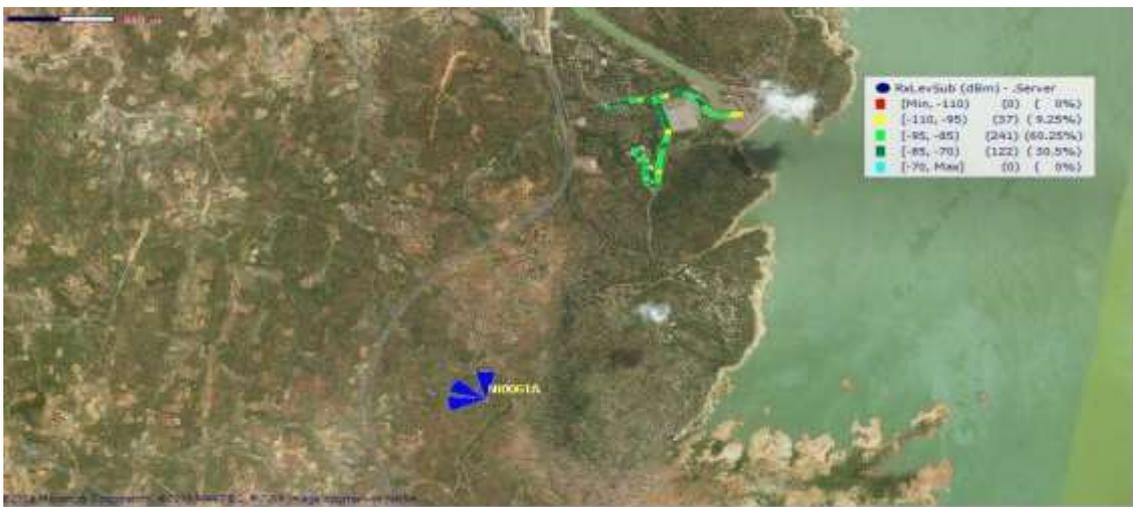
Figure 4.5: The received signal strength for Network C
