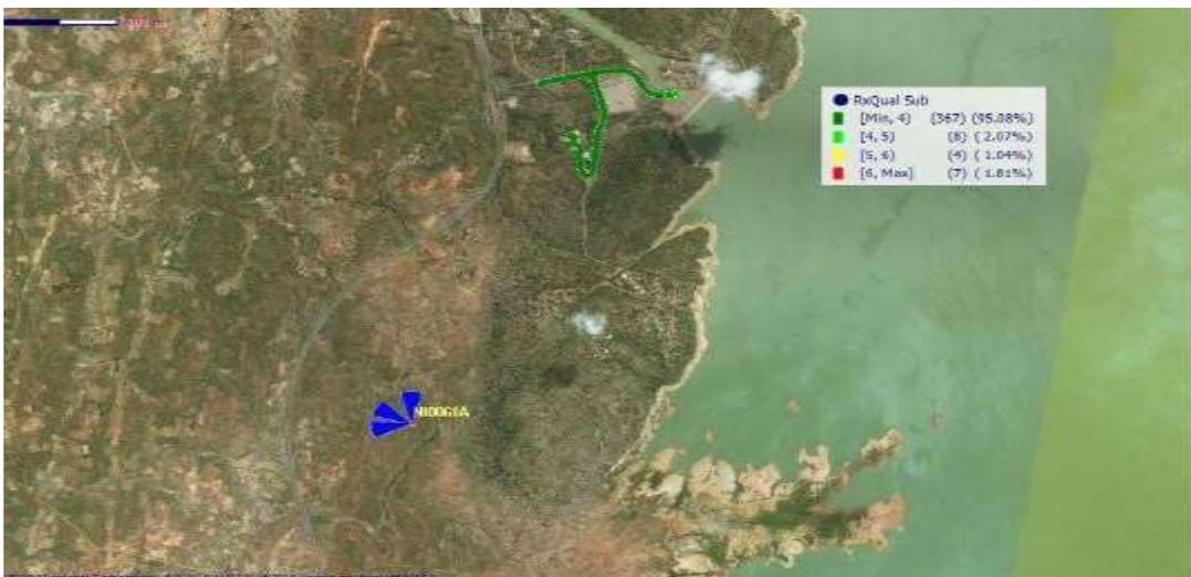
Figure 4.6: The received voice quality for Network C
