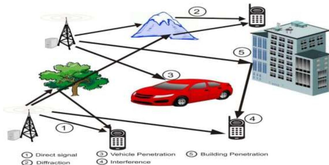
**Figure 2.2: Factors affecting wave propagation (Aliyu *et al.*, 2018).**
