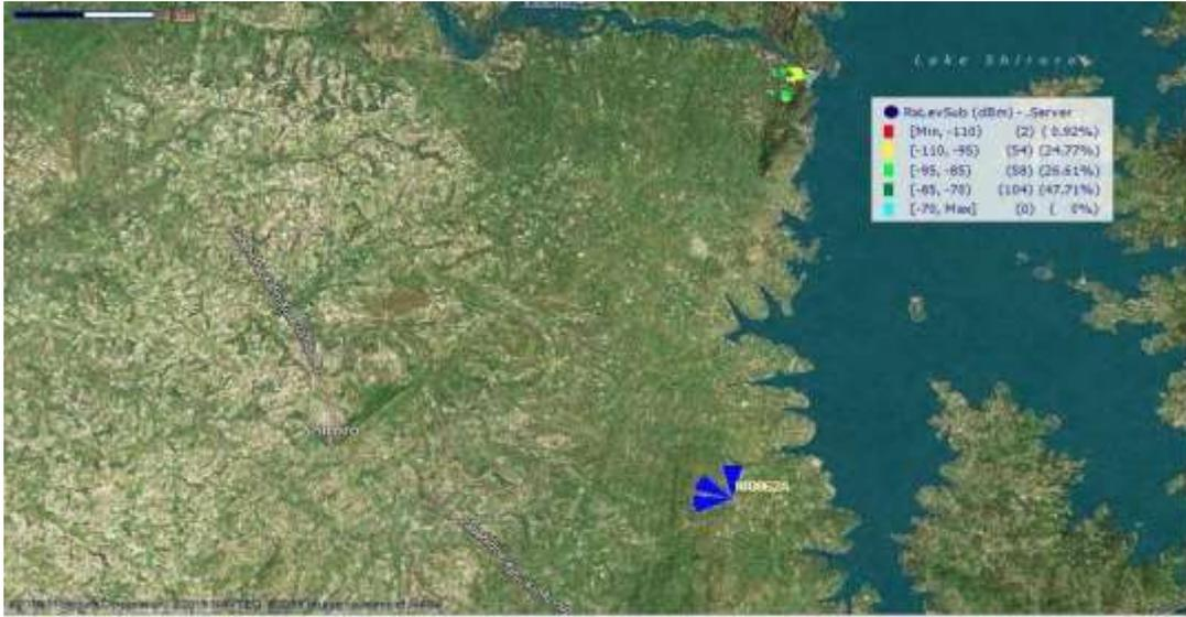
Figure 4.3: The received signal strength for network B
