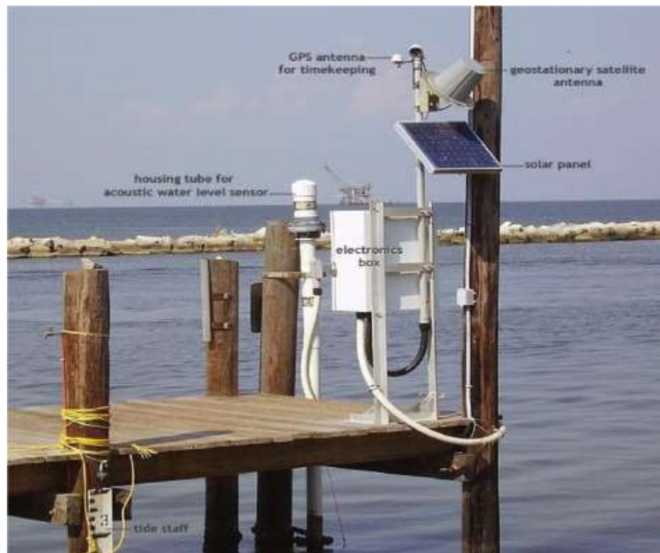
Plate I: An Automatic Tide Gauge (NOAA, 2019)
