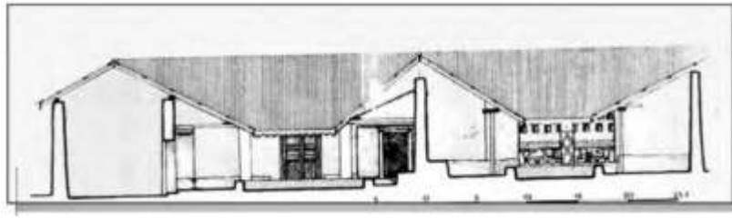
Fig 2.6: A section of courtyard house showing threshold and floor level difference. Source: (Dmonchowski, 1990)
