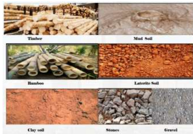
Plate XII: Shows materials that defines Yoruba Traditional Housing Source: (Author's field work, 2021)
