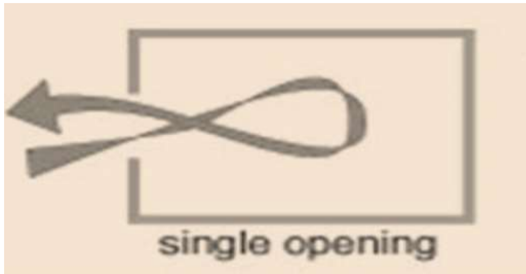
Figure 2.13: Single Sided ventilation air flow Source: Ghiaus et al. (2005)
