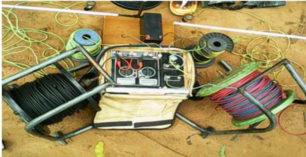
Plate IIIb: Acquisition of electrical resistivity data on field using a rectified terrameter.
