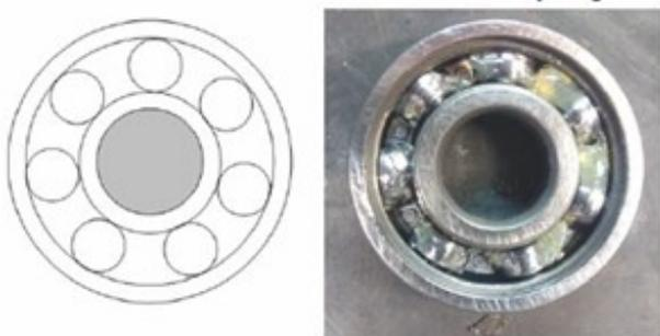
Figure 1: Diagram and plate of a healthy bearing [3].
