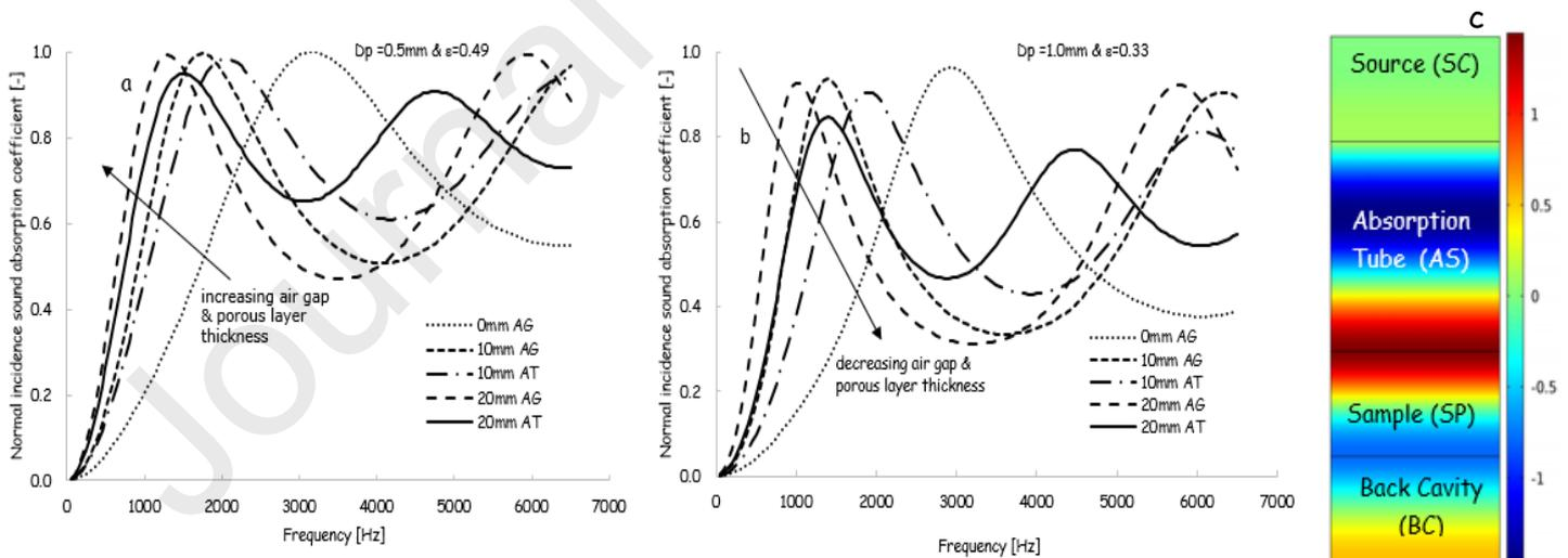
Fig 6. Plots of dimensionless numerically simulated normal incidence sound absorption coefficient for increasing air gap (back cavity) and porous layer thickness for optimally selected pore-related parameters (a) Particle size,  $0.5 \text{mm}$  & void fraction,  $0.49$  and (b) particle size,  $1 \text{mm}$  & void fraction,  $0.33$ . Fig 6c. Plot of total acoustic pressure of 2D incidence plane wave on porous sample supported with an air gap or back cavity.
