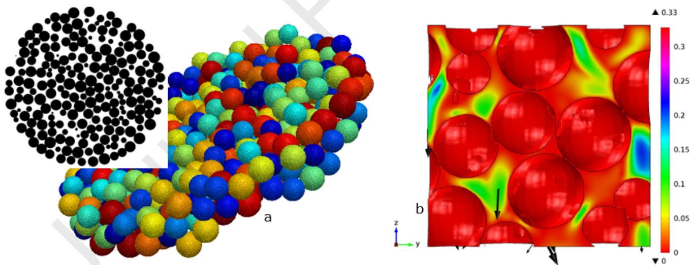
Fig 1. (a) Left of velocity ( $\text{m.s}^{-1}$ ) streamline/arrow plots of flowing fluid across representative packed spheres is a two- and three-dimensional images of virtual macroporous packed spheres characterised by particle size 2.0mm and 0.33 void fraction.
