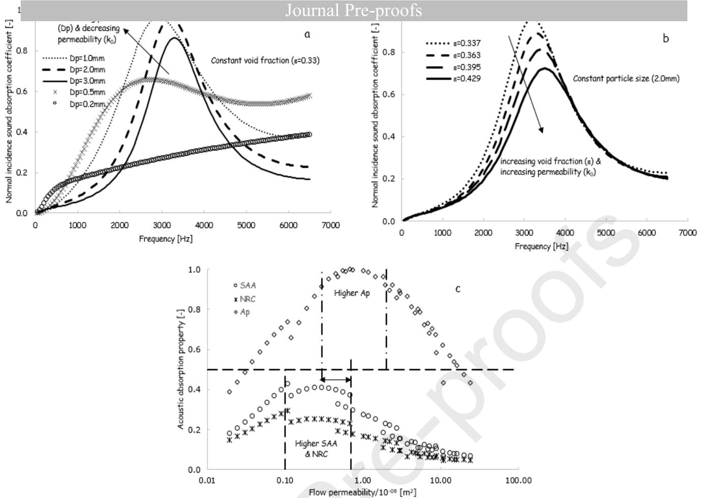
Fig 5. Plots of the dimensionless numerically simulated normal incidence absorption coefficient for varying (a) particle size and (b) pore volume or void fraction while (c) represents plots of predicted sound absorption properties against flow permeability for particles in the range of 0.2 - 4.0mm and void fractions between 0.33 and 0.49.
