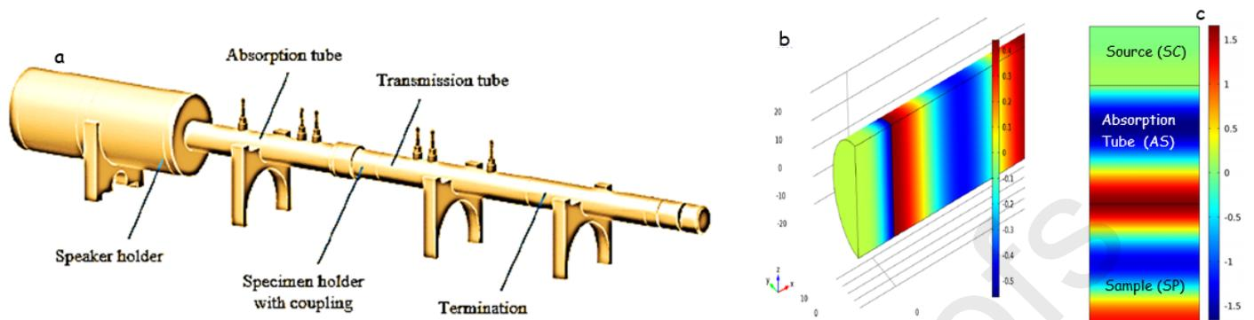
Fig 2. (a) An AFD 1200-AcoustiTube® (adapted from [Otaru, 2019b; Otaru et al, 2018]), (b) Three-dimensional half-tube and (c) two-dimensional numerically simulated total acoustic pressure for 20mm hardbacked packed spherical structures.
