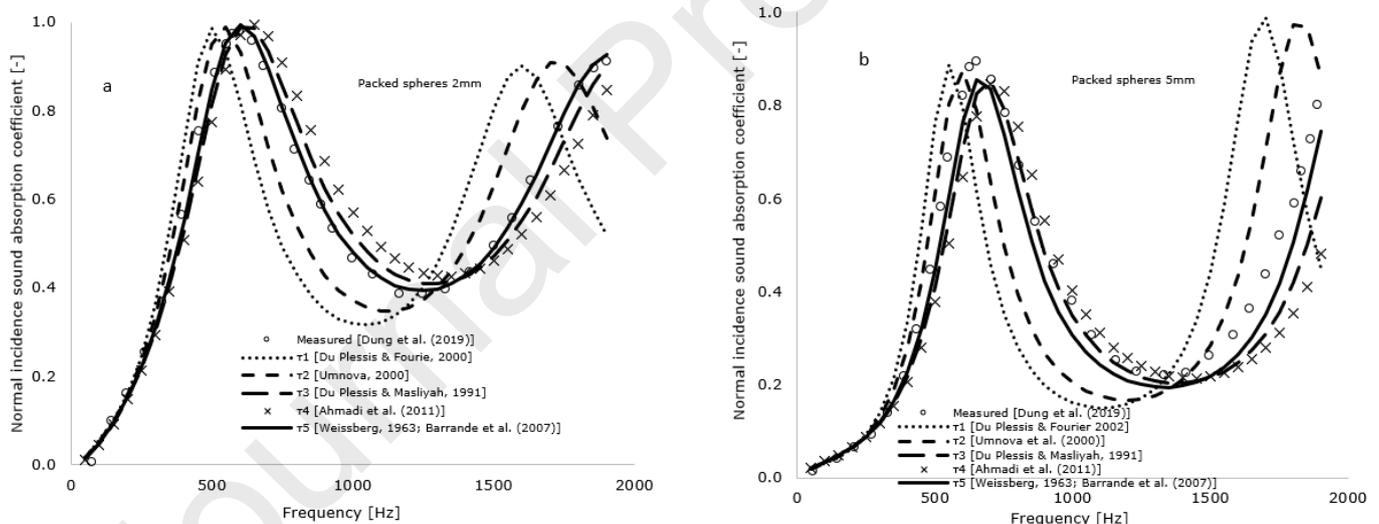
Fig 4. Plots of the dimensionless numerically simulated normal incidence absorption coefficient using different tortuosity ( $\tau_i$ ) predictive models against experimentally measurements (Dung et al., 2019) for packed spheres characterised by (a) 2mm and (b) 5mm mean particle size.
