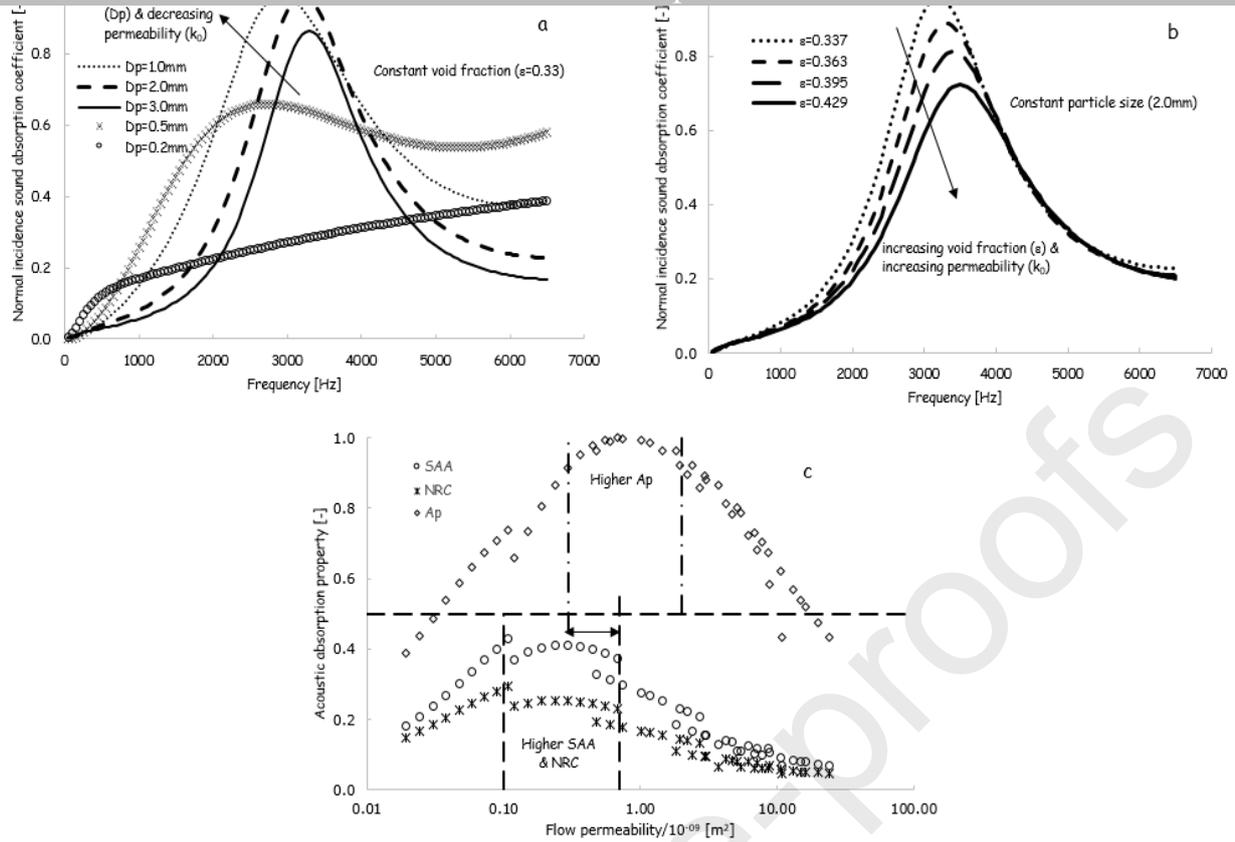
Fig 5. Plots of the dimensionless numerically simulated normal incidence absorption coefficient for varying (a) particle size and (b) pore volume or void fraction while (c) represents plots of predicted sound absorption properties against flow permeability for particles in the range of 0.2 - 4.0mm and void fractions between 0.33 and 0.49.
