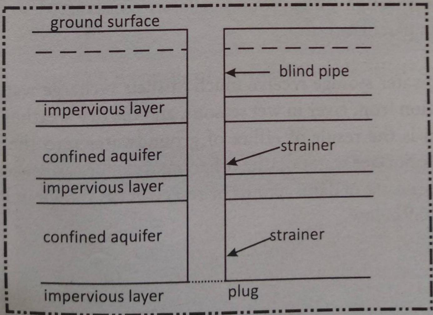
Fig. 10.1 Strainer type of tube well
