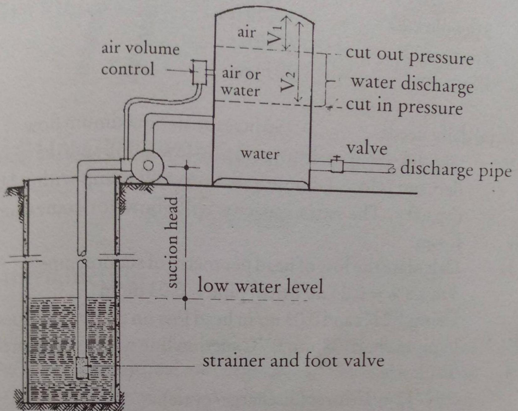
Fig. 10.2 Hydro pneumatic water system
