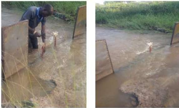
Figure 2: Weir Installation and runoff measurement
