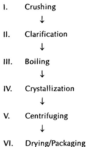
**Fig. 1. : Flow chart for sugar extraction from sugarcane**
