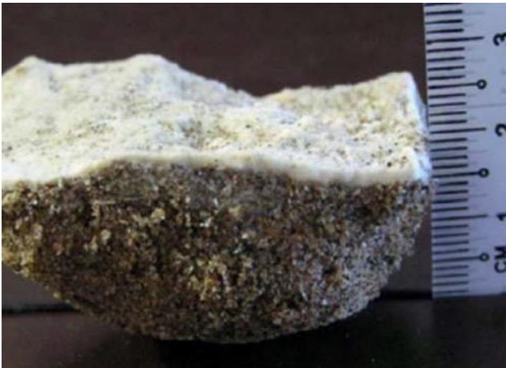
**Figure 1.7: 1mm thick calcite crust formed on the surface of the soil(Noshi and Schubert, 2018).**
