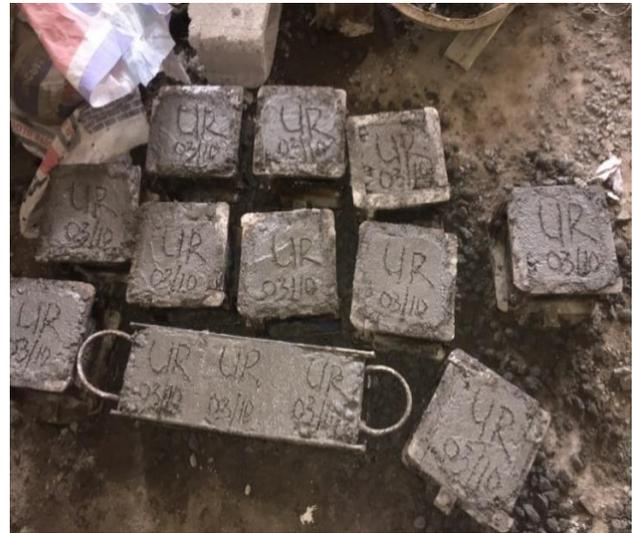
Plate I: Concrete cubes cast with 0 % urease Plate II: Concrete cubes cast with (80 %) urease
