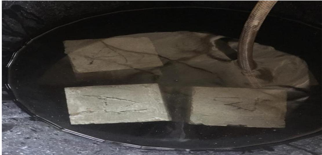
Plate III: Concrete cubes cured in curing tank
