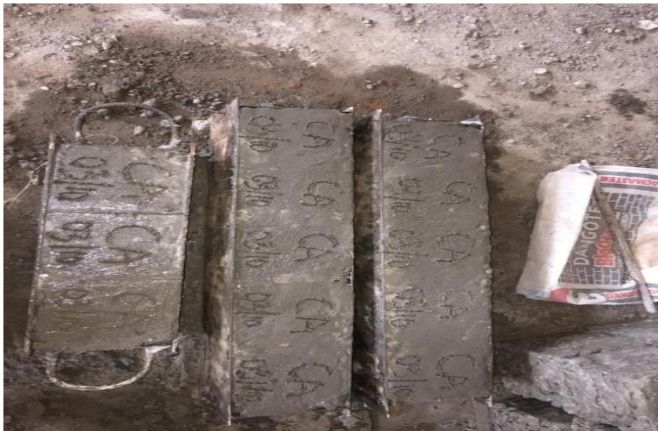
Plate II: Moulded concrete cubes
