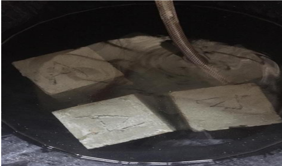
Plate III: Curing of demoulded concrete cubes
