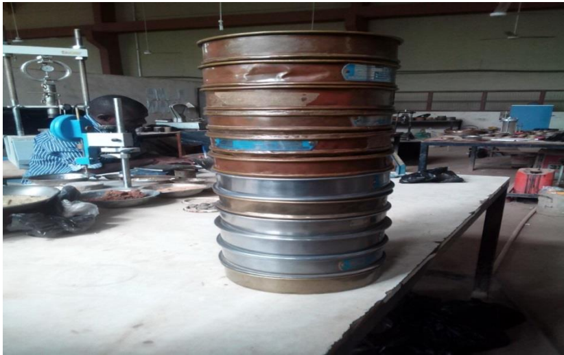
Plate I: Set of sieves for particle size distribution
