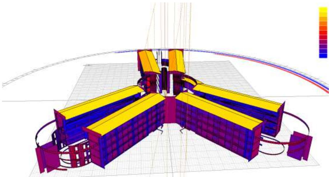
**Figure 4. 10 Solar access radiation on building elements**
