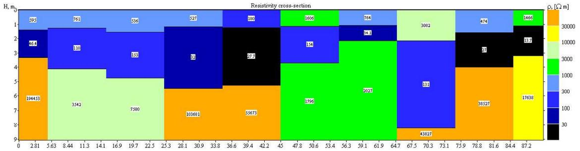
Figure 2c: Geo- electric Section for Transverse I
