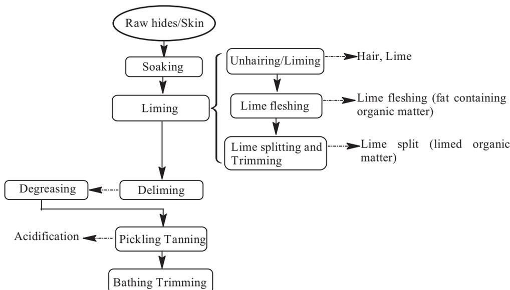
Fig. 1. A schematic diagram of the tanning process.
