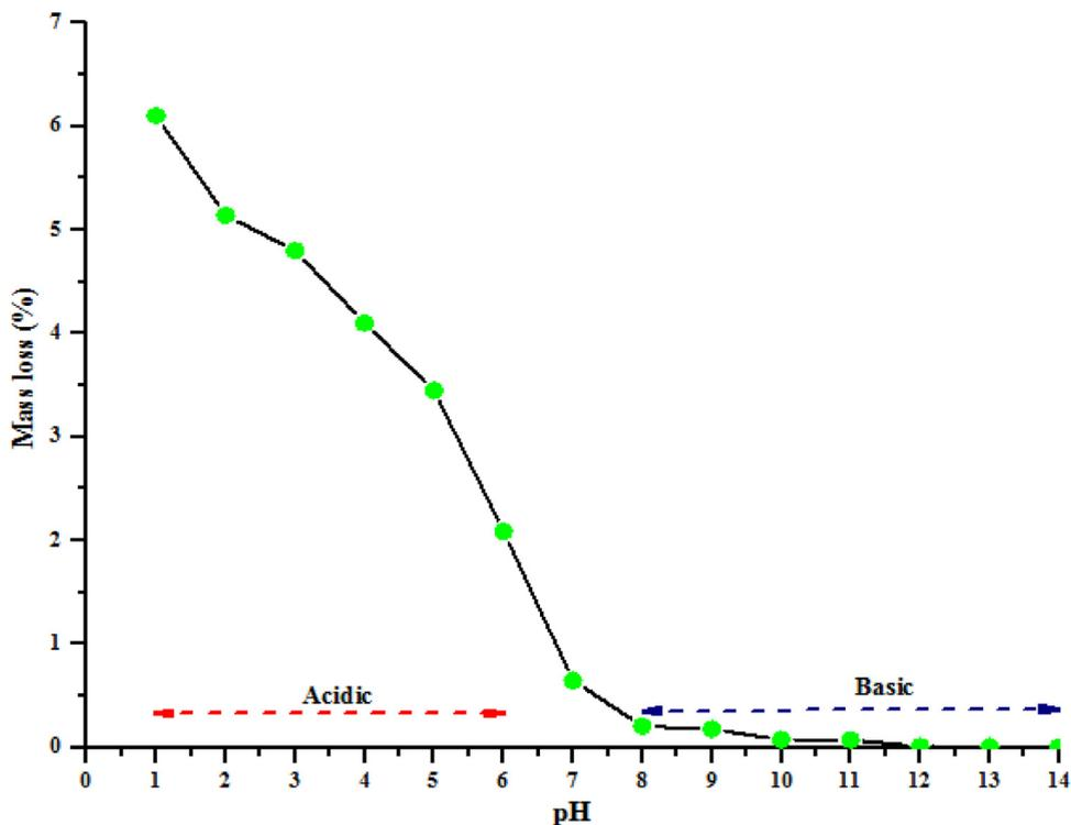
Fig. 9. Weight loss (%) of optimal sintered kaolin/sawdust filter inacidic and basic medium at ambient temperature for 48 h.
