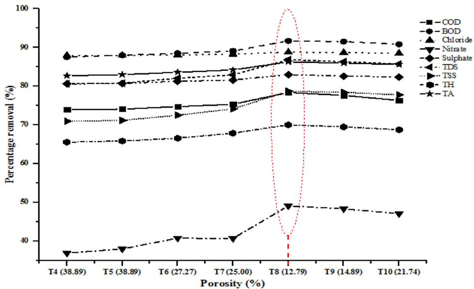
Fig. 6. The total removal efficiencies of the regular pot filters.
