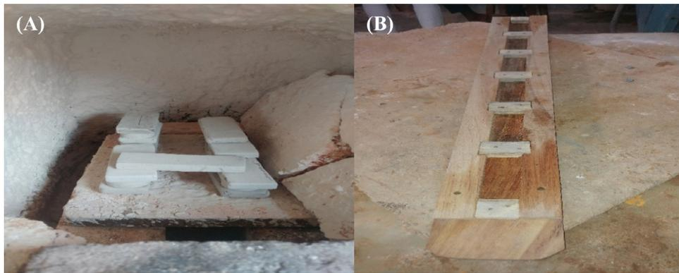
**Plate 1.** (A) Trial bars prepared from beneficiated kaolin and (B) Mould.
