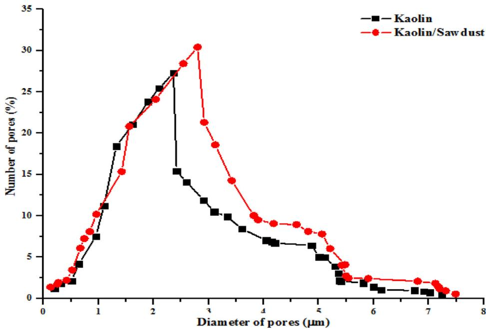
Fig. 5. Pore size distribution of kaolin and kaolin/sawdust sinter at 910 °C.
