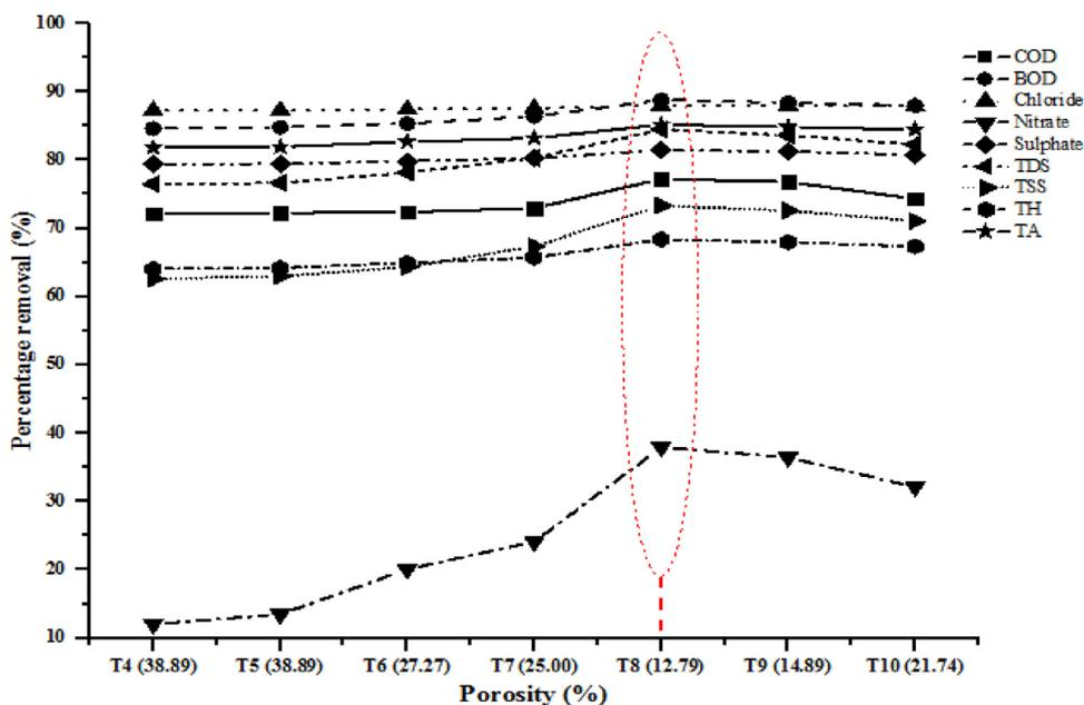
Fig. 8. The total removal efficiencies of the second scrubbed pot filters.
