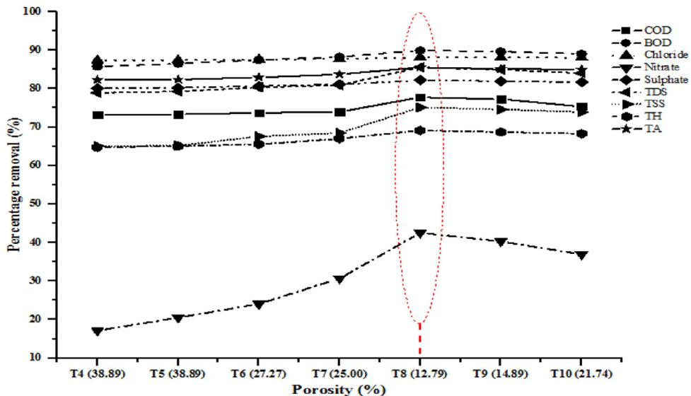
Fig. 7. The total removal efficiencies of the first scrubbed pot filters.
