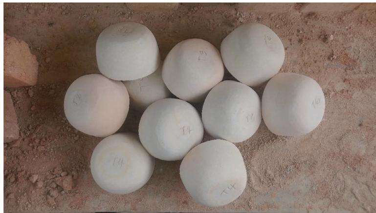
**Plate 4.** Fabricated kaolin pot filters at different proportions of sawdust and kaolin
