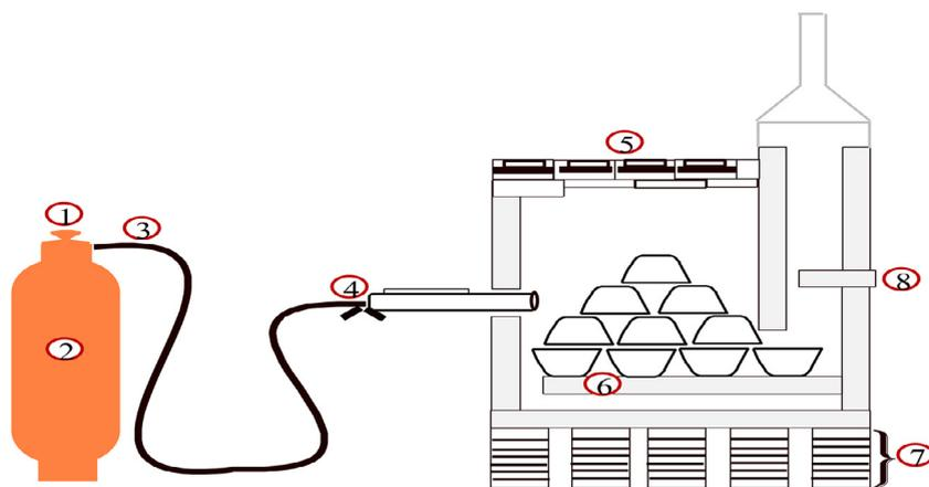
1. Tap 2. Gas cylinder 3. Nozzle 4. Burner 5. Roof parts 6. Internal floor 7. Pillars 8. Chimney
