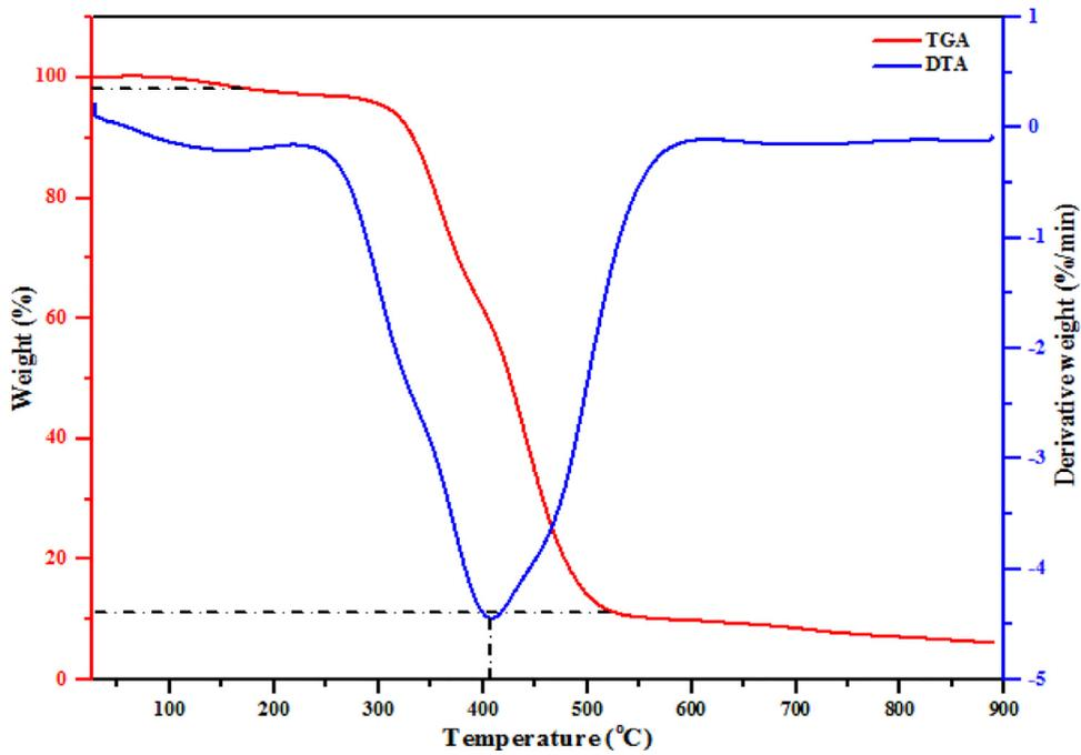
Fig. 4. TGA/DTA of kaolin/sawdust calcined at 910°C.
