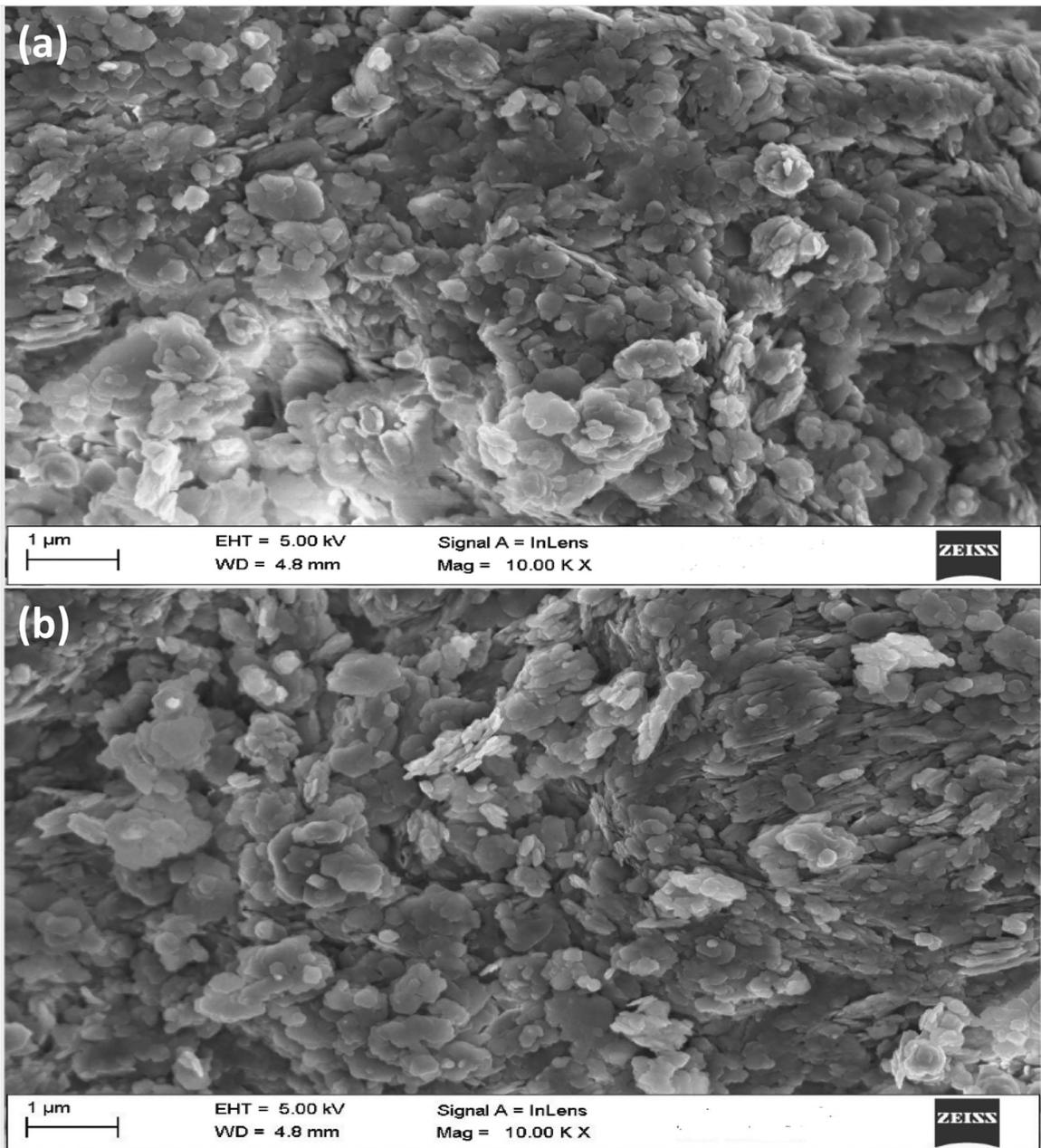
**Plate 3.** HRSEM microimages of kaolin (a) and compacted pellet of kaolin/sawdust (b) sintered at 910 °C.
