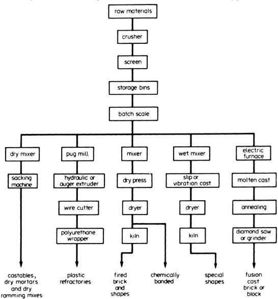
Fig.3.2: Schematic of the processes used in the manufacture of refractory products
