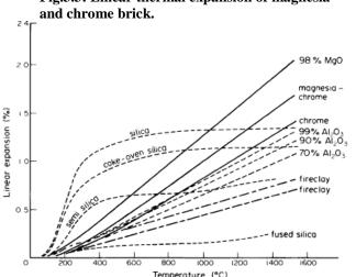
Fig.3.3: Linear thermal expansion of magnesia
