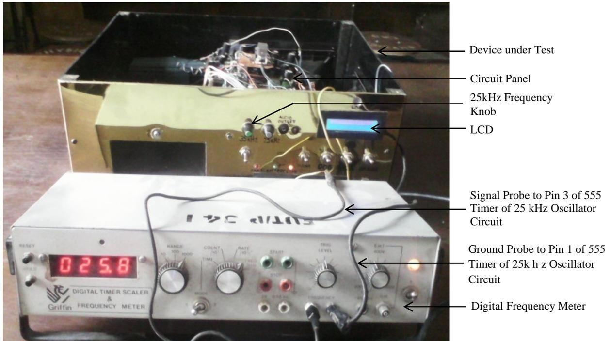
Plate IV: Frequency Meter Readout of the 25 kHz Oscillator
