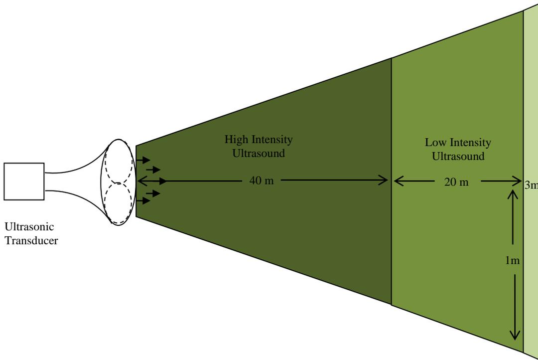
Figure 1: Illustration of Ultrasonic Transducer's area of coverage
