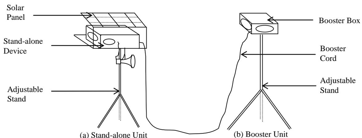
Figure 1: Schematics of the Ultrasound Booster System
