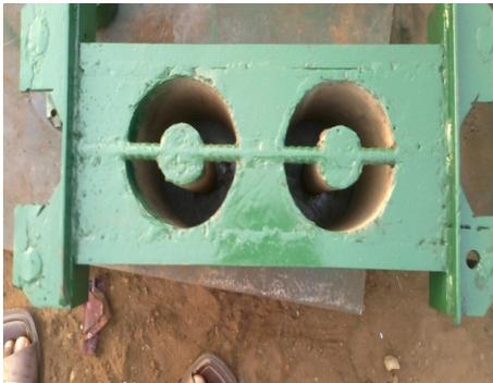
**Plate 3.** Machine mould unit.
