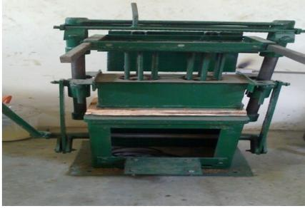
**Plate 1.** Motorized vibratory briquette making machine.
