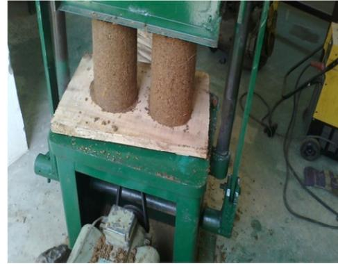
Plate 7. Ejection of briquettes from machine.
