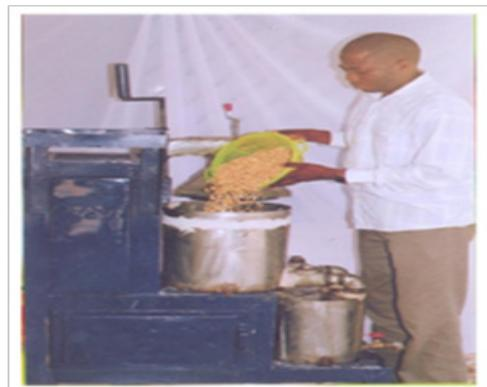
Figure 5 Feeding of grains into the machine.
