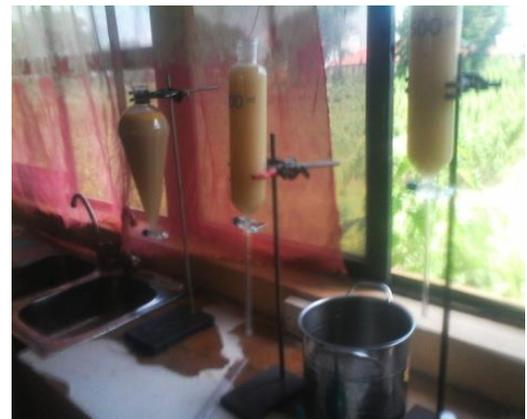
Plate i Showing oil and water separation technique
