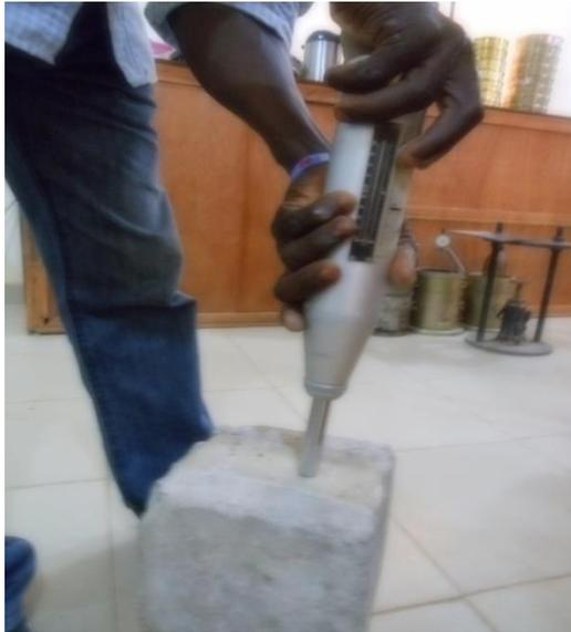
Plate I: Testing Using Schmidt Rebound Hammer
