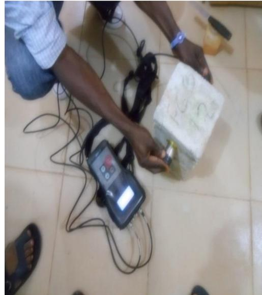
Plate II: Testing Using UPV Machine
