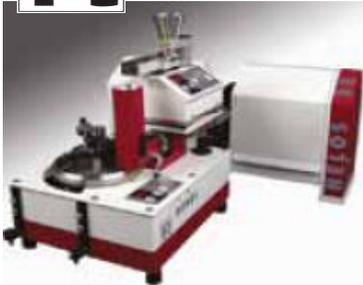
Laser Diffraction Particle Size Analyser
