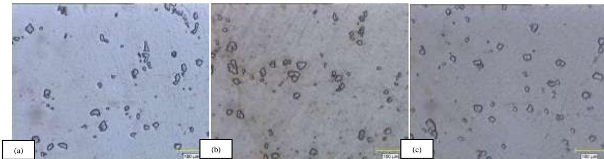
Figure 11) microstructure of different alloys after double solution treatment a) hafnium free alloy, b) 0.6 wt pct added hafnium alloy, c) 1.5 wt pct added hafnium alloy
