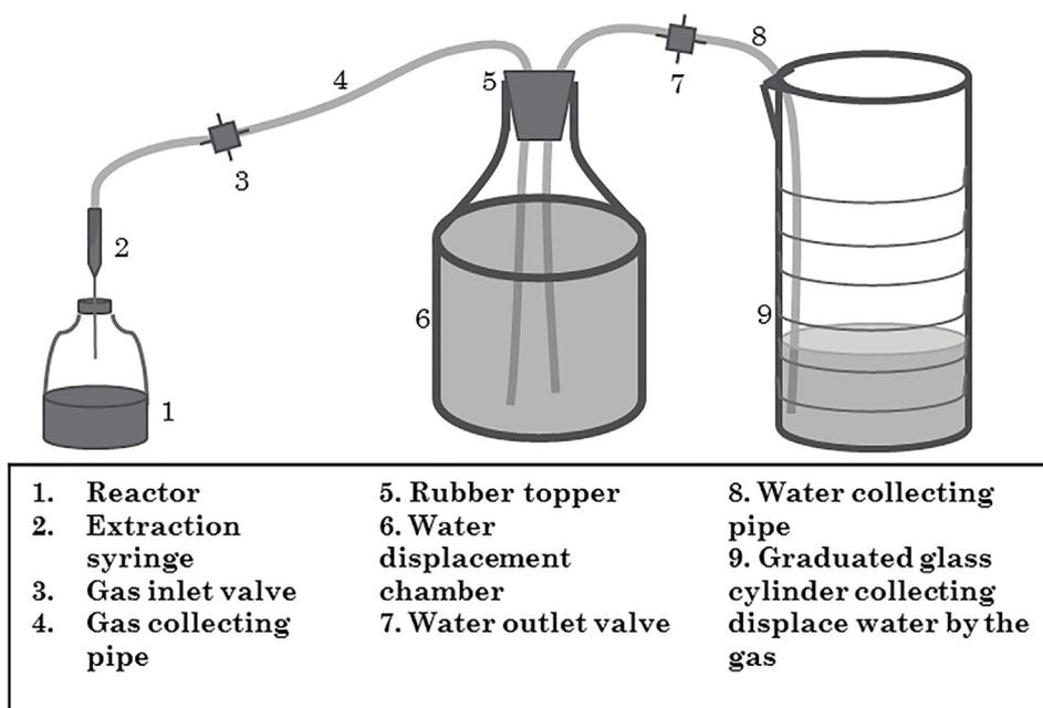
Fig. 2. Schematic setup for headspace gas volume measurement by water displacement.
