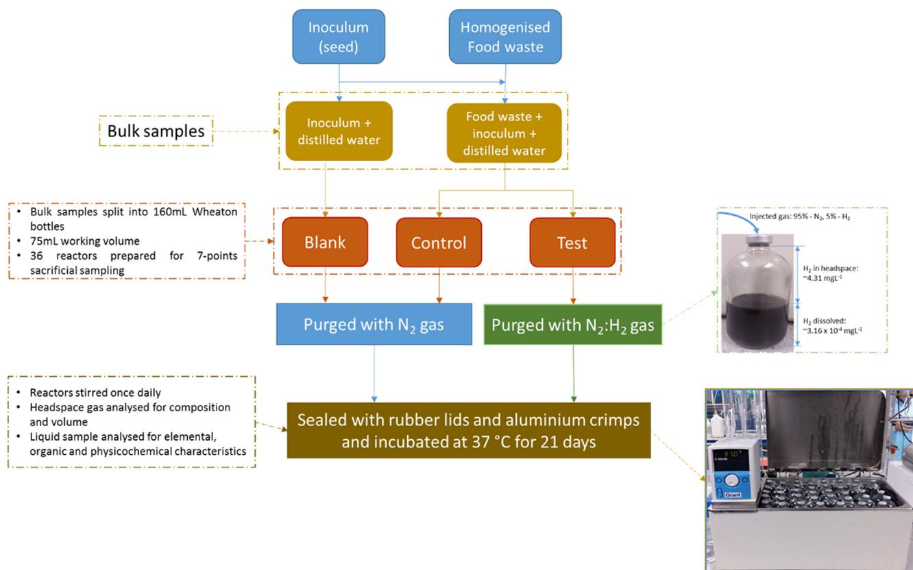
Fig. 1. Experimental setup showing the preparatory stages for anaerobic digestion with hydrogen addition.
