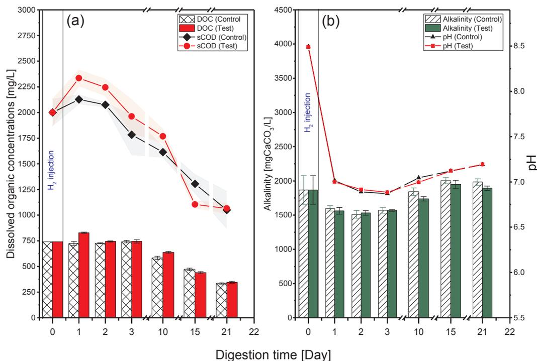
Fig. 5. (a) Dissolved organic concentrations (sCOD and DOC) in the reactors. Shaded areas in sCOD plots indicate error margin based on standard deviations from mean; (b) Alkalinity (column graphs) and pH pattern during the experimental period.
