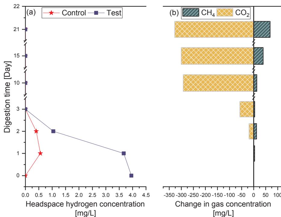
Fig. 3. (a) Hydrogen concentration in the headspace of the control and test reactors and (b) Change in CH<sub>4</sub> and CO<sub>2</sub> concentration, taken as difference between concentrations from test and control reactors (e.g., CH<sub>4</sub> test – CH<sub>4</sub> control).
