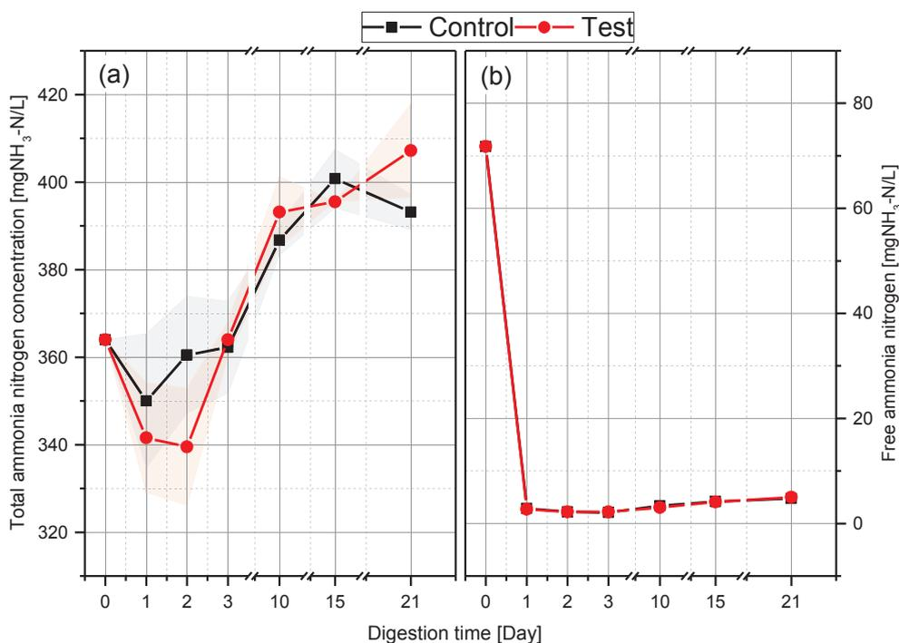
Fig. 6. Ammonia-nitrogen concentration; (a) total ammonia nitrogen (TAN), where shaded portion indicates magnitude of standard deviation from the mean, (b) free ammonia nitrogen (FAN) calculated from the corresponding TAN and pH using formula detailed in [42].
