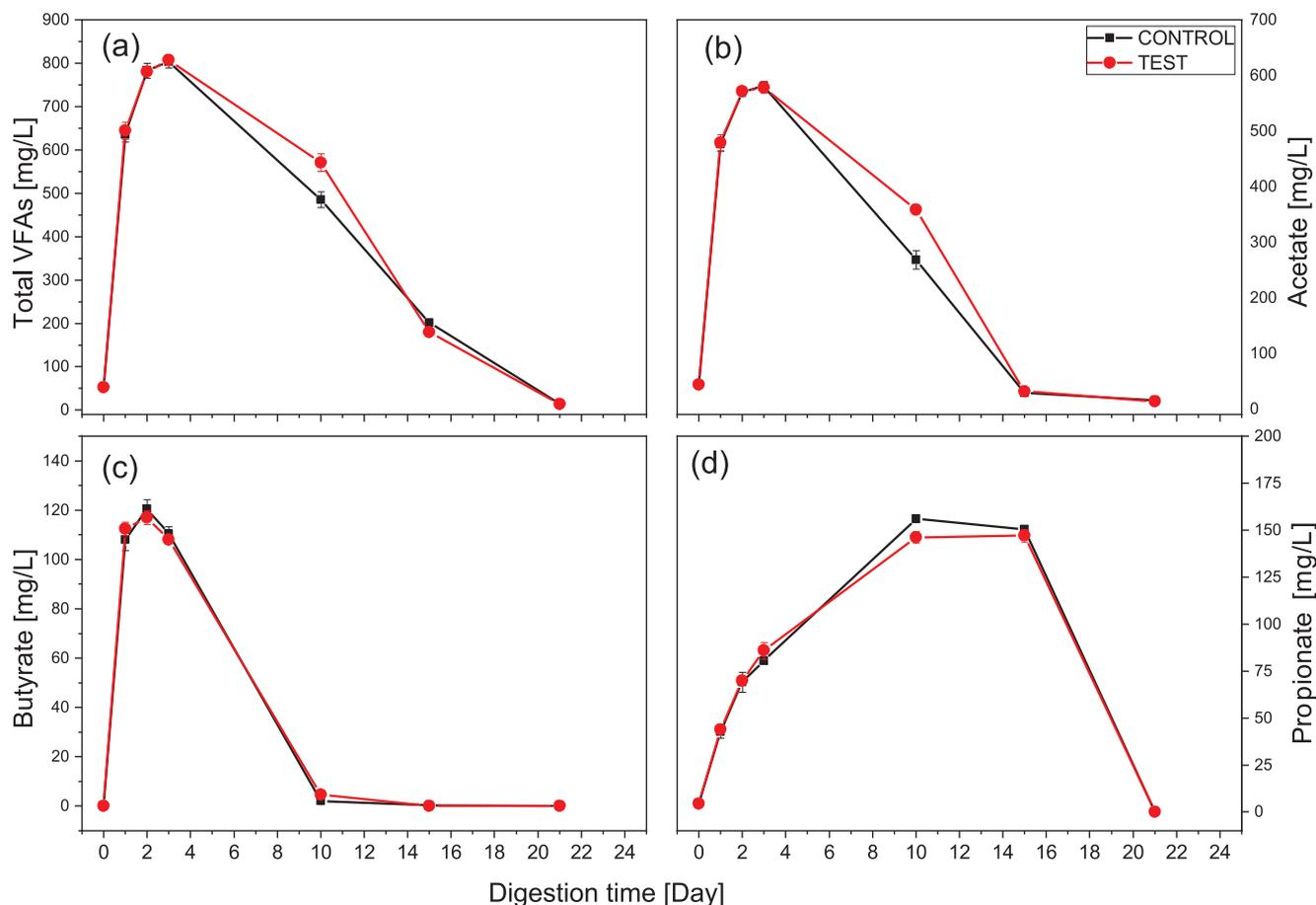
**Fig. 4.** VFA concentrations comparison between the test and control reactors. Error bars are the standard deviation from the mean.
